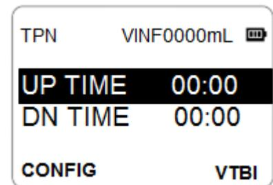
The TPN infusion parameters may be programmed by using the UP/DOWN Arrow keys and Data Entry keys.
