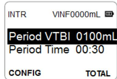
The Period VTBI and Period Time parameters may be programmed by using the UP/DOWN Arrow keys and Data Entry keys.
