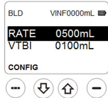
The RATE and VTBI parameters may be programmed by using the UP/DOWN Arrow keys and Data Entry keys.
