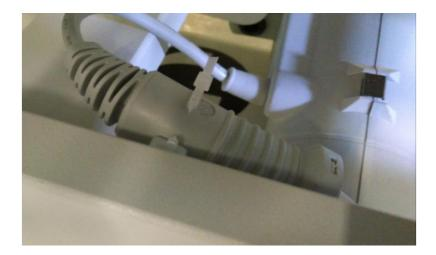
• Remove the protection by pressing a flat screwdriver between the socket and the lock, remove the plug.
