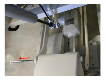
• Remove the protective sheath and circlip from the lower axis of actuator, then knock out the axle.
