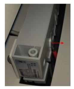
• Remove the lock and romove the cables.
