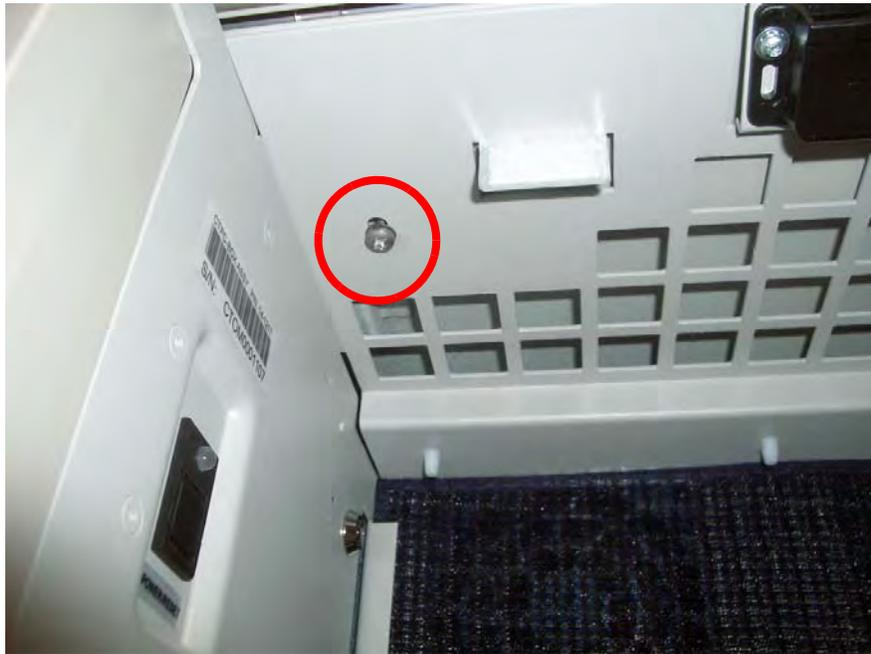
**Figure 1-9.** Add the M4x14 security screw
