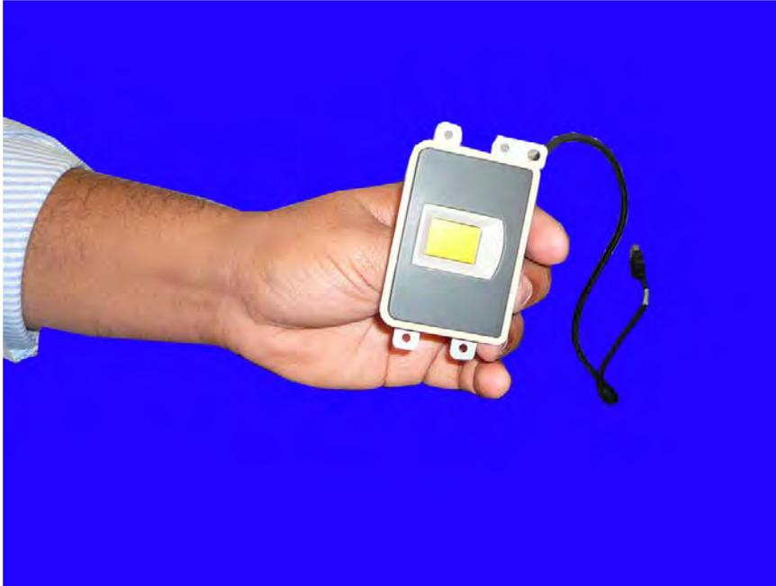
**Figure 3-4.** Ensure the gasket is secure
