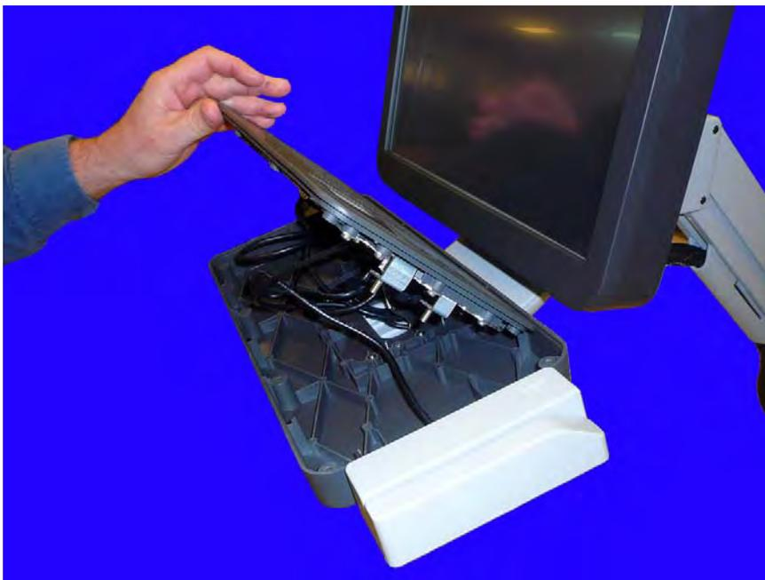
**Figure 3-3.** Lift the keyboard from the keyboard enclosure
