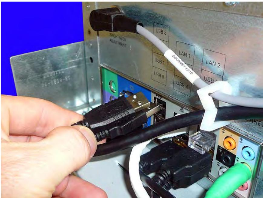
**Figure 1-8.** Plug the USB cable(s) into the USB ports
