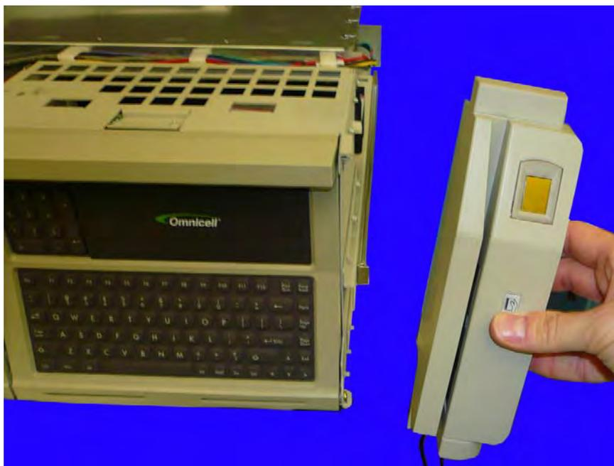
**Figure 1-3.** Put the card reader and fingerprint scanner in place
