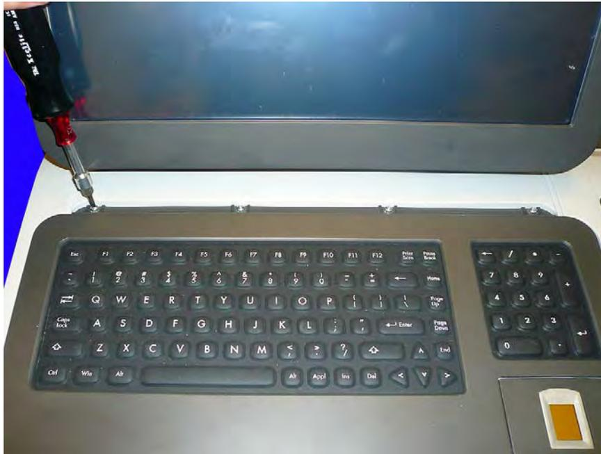
**Figure 2-2.** Remove the top four screws that secure the keyboard
