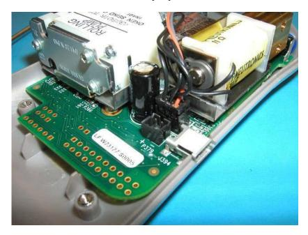
4. Remove the 2 screws that secure the electro-mechanical assembly to the PCB, one will be hidden under the left side of the manifold.
