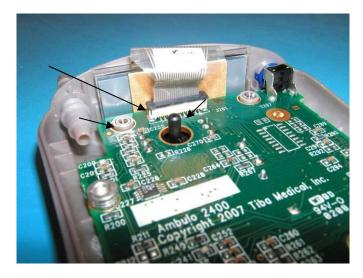
7. Remove the 2 screws that connect the PCB to the top cover. You can now remove the PCB from the device.
