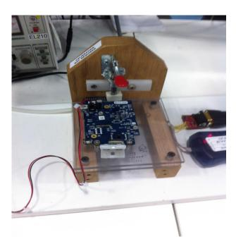
2. The input of the pressure transducer should be connected to a calibrated pressure source (attach the tubing to the pressure port as below).
