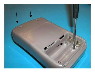
2. Carefully lift the bottom cover and disconnect the Hirosi-terminated battery connector from the PCB. You can now remove the bottom cover from the device.
