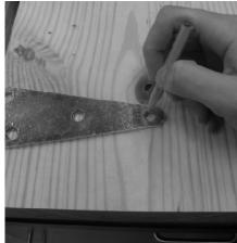
3. Use a tape measure or ruler to draw a straight line between the holes. This line must be parallel to the edge of the wood.
