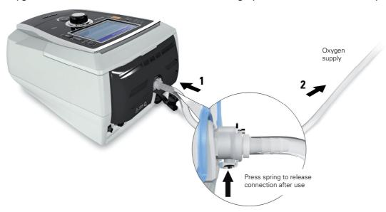
Note: Up to 30 L/min at maximum oxygen pressure of 50 mbar (0.73 psi) can be added.
