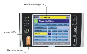
Alarm messages are displayed along the top of the screen. High priority alarms are displayed in **red**, medium priority alarms in **yellow** and low priority alarms in **light blue**. The Alarm LED lights **red** during high priority alarms and **yellow** during medium and low priority alarms.
