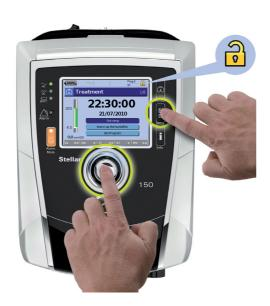
To activate Clinical mode ①, hold down and I simultaneously for at least three seconds. You will be prompted for how long the device should stay in this mode. After the set period of inactivity or next power cycle (power on/off), the device automatically switches back to the patient mode and the device beeps.
