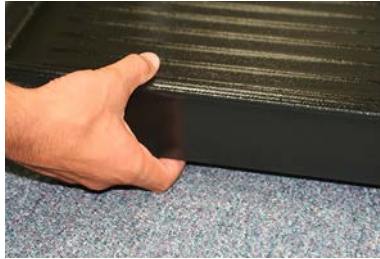
Figure 2-2. Clearance Between Scale Base and Floor
