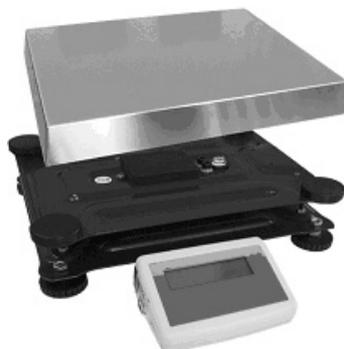
Level balance with foot screws until the air bubble of the water balance is in the prescribed circle.
