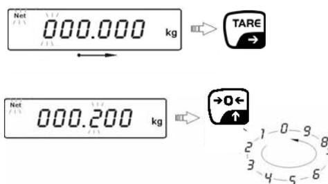
⇒ Select the point to be changed by pressing the button and the number by pressing the button and the active point flashes in each case.
