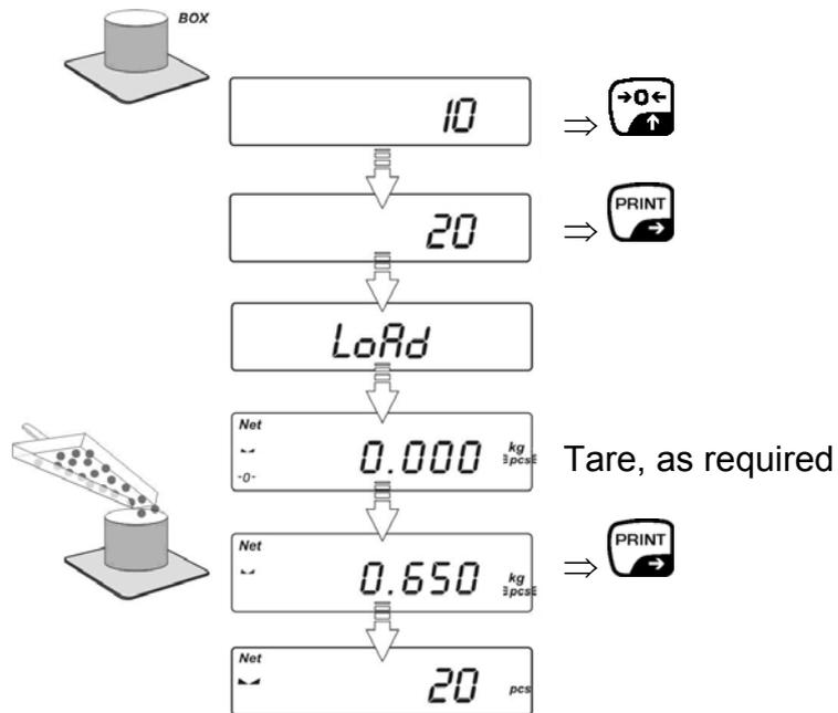
Remove reference weight. The balance is now in parts counting mode counting all units on the weighing plate.
