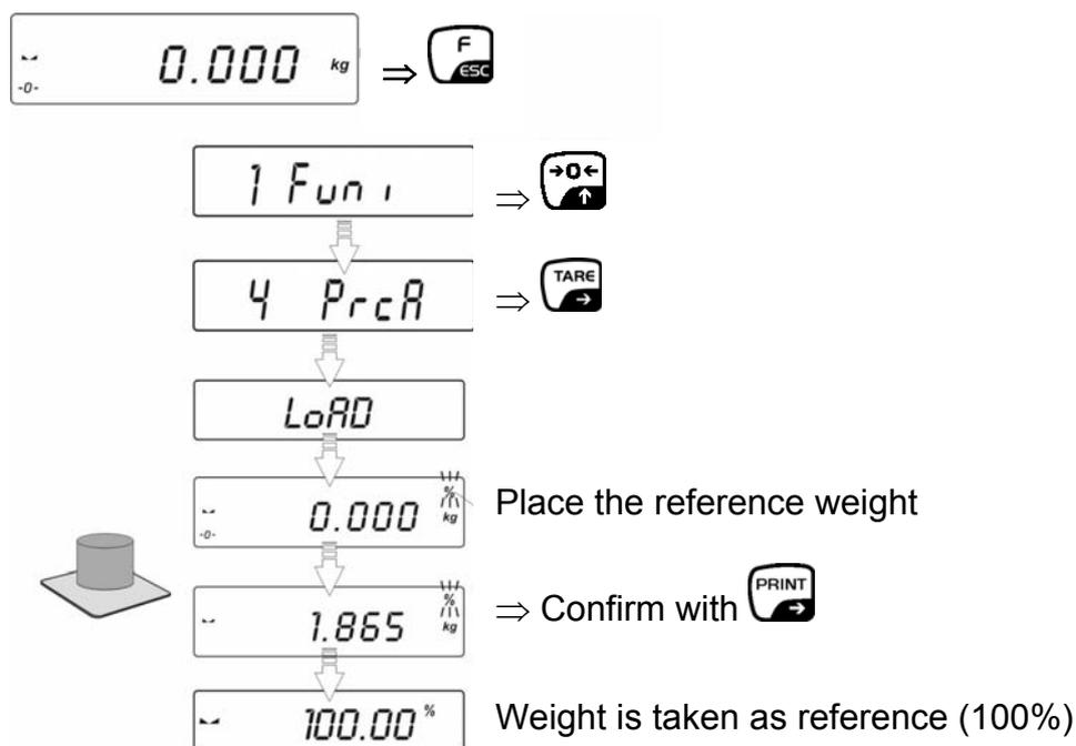
Remove reference weight. The balance is now in percent determining mode. Place the load on the balance; percentage value in relation to reference body is shown on display:
