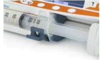
5. Squeeze the finger grips on the plunger holder and slide the mechanism to the left until it reaches the plunger end.
