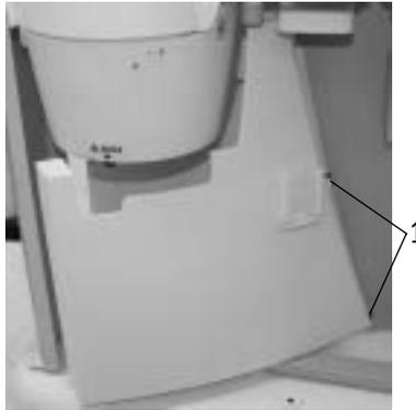
3. Loosen the thumbscrew and remove the reservoir (2). It is not autoclavable.
