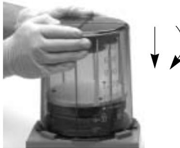
7. In the above steps, if you see a dust-like powder on the bellows housing or on the bellows, apply a thin layer of KRYTOX lubricant to the ribs of the bellows housing. Make sure the lubricant is applied smoothly and there are no lumps.
