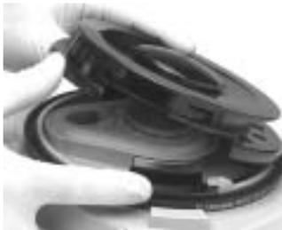
5. Attach the bottom edge of the bellows to the rim. Verify only the bottom ring of the bellows is fitted over the rim.
