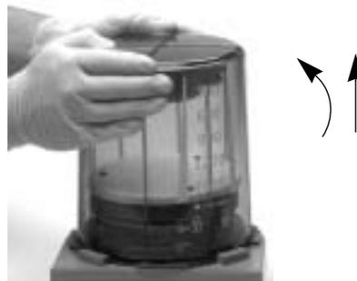
2. Remove the bottom edge of the bellows from the rim.
