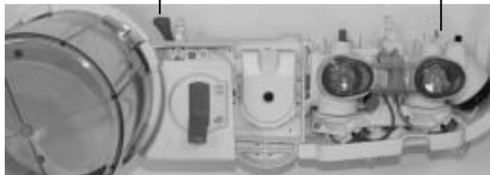
3. Holding the rear handle (1) and the latch handle (2) as shown, slide the breathing system onto the guide pins.
