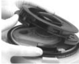
4. Remove the pressure-relief valve.
