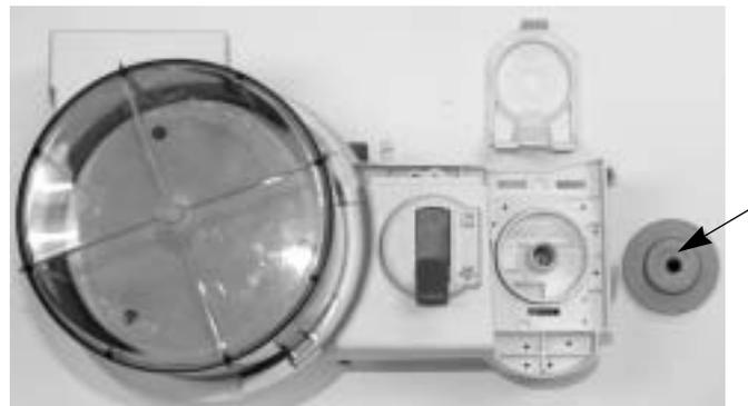
11. Turn over the bellows base assembly, grasp the bellows boot with three fingers in the openings at the points shown and pull straight away to remove it.
