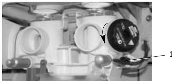
5. Remove the flow sensors from the module:
