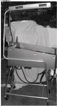
In the resistance element, long rods are placed approximately 1 meter above the level of the infant, reflecting heat downwards. There is an open grille that covers the rods. When energized the rods glow red. Some old versions may use open coils, which can give inconsistent heat distribution over the infant.
