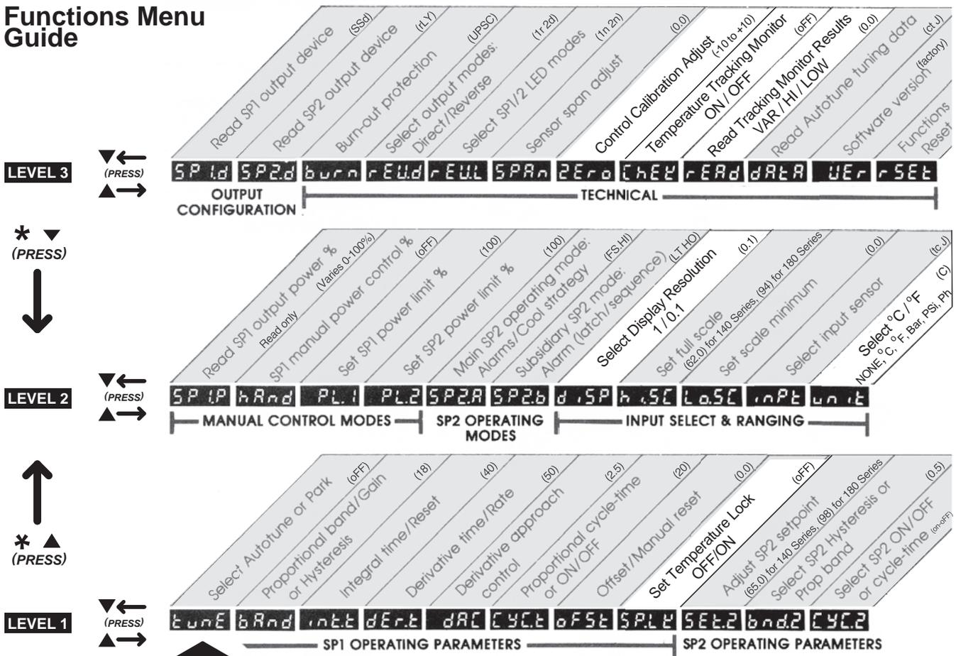
**IMPORTANT NOTE:** The grey-shaded control functions within the menu levels are factory tuned and set for the optimum performance and the safe operation for your model incubator. Care should be taken when navigating or changing user applicable settings so as not to alter these factory settings. Factory settings for each function are listed within the parentheses "( )" on each function tab above. Use as a trouble-shooting reference.
