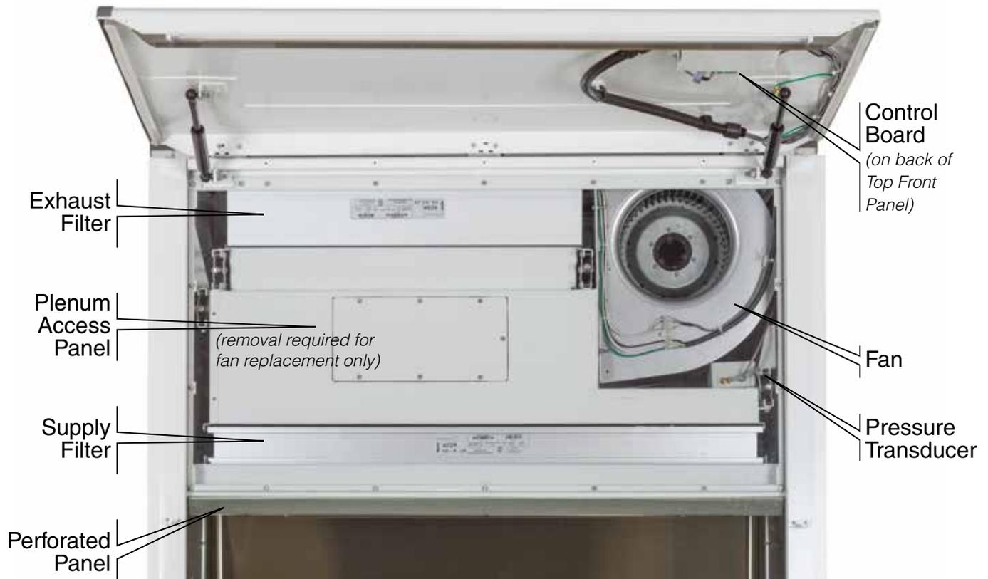
Figure 2.2 BSC with Air Chamber Access Panel removed
