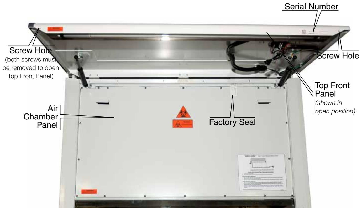
Figure 2.1 BSC with Top Front Panel open
