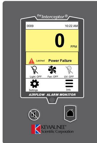
Figure 4.3 Home/Face Velocity Screen - Latched/Power Failure
