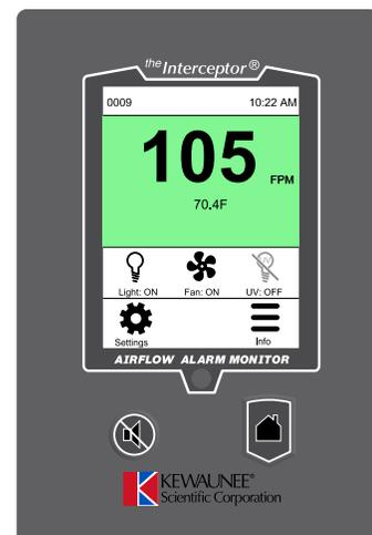
Figure 4.6 Home/Face Velocity Screen - Safe Operating Condition
