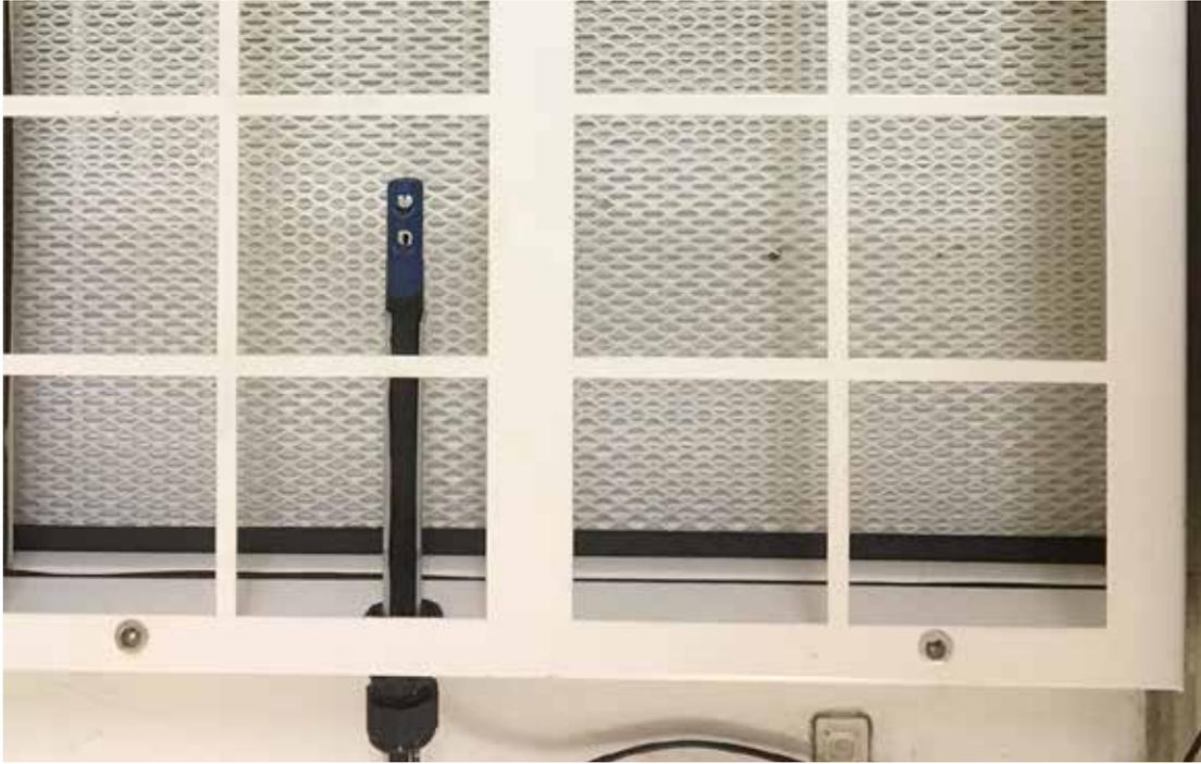
Figure 3.5 Face Velocity Sensor
