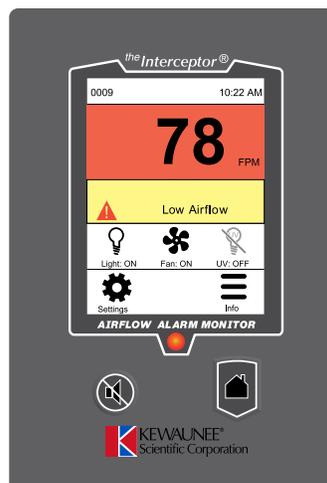
Figure 4.5 Home/Face Velocity Screen - Fan Warm-Up
