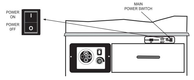
Figure 4-1. Control Panel Main Power Switch Location
