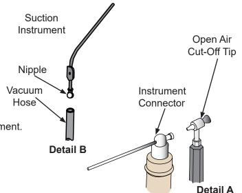
Figure 4-11. Instrument Attachment
