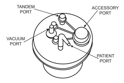
Figure 5-2. Replacing the S 740600C Disposable Canister Liner
