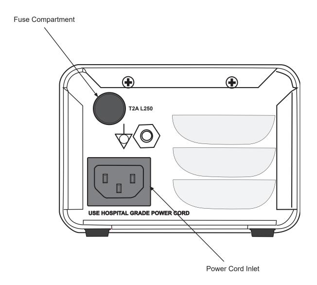
Figure 5-5. S 740200LED Light Source Back Panel
