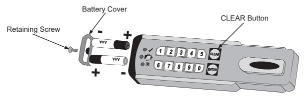
Figure 5-6. Replacing Batteries in the Keyless Locking System
