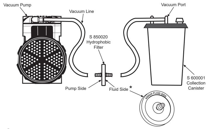
(I)NOTE The side of the filter marked "FLUID SIDE" should always face towards the collection canister.
