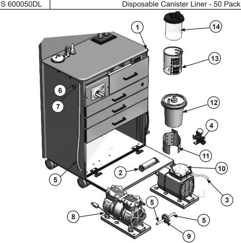
Figure 7-1. Pump Compartment Component Breakdown
