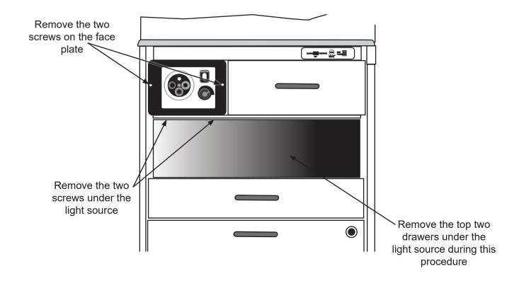
Figure 5-4. Replacing the S 740200LED Light Source Fuse
