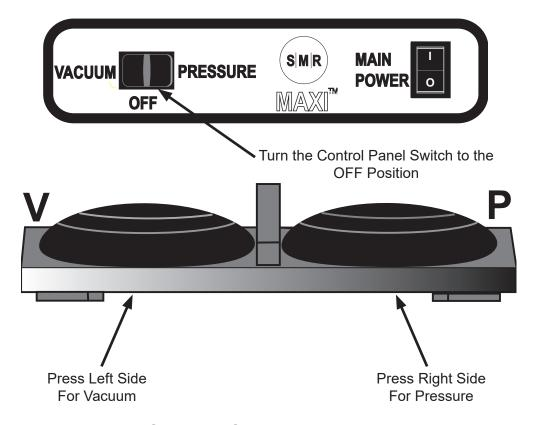
Figure 4-9. Optional S 7401355 Suction / Pressure Foot Switch Operation
