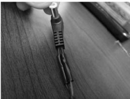
10. Plug the transformer into the wall. Test for the voltage output with the multimeter. The voltage output should be the desired output. .
