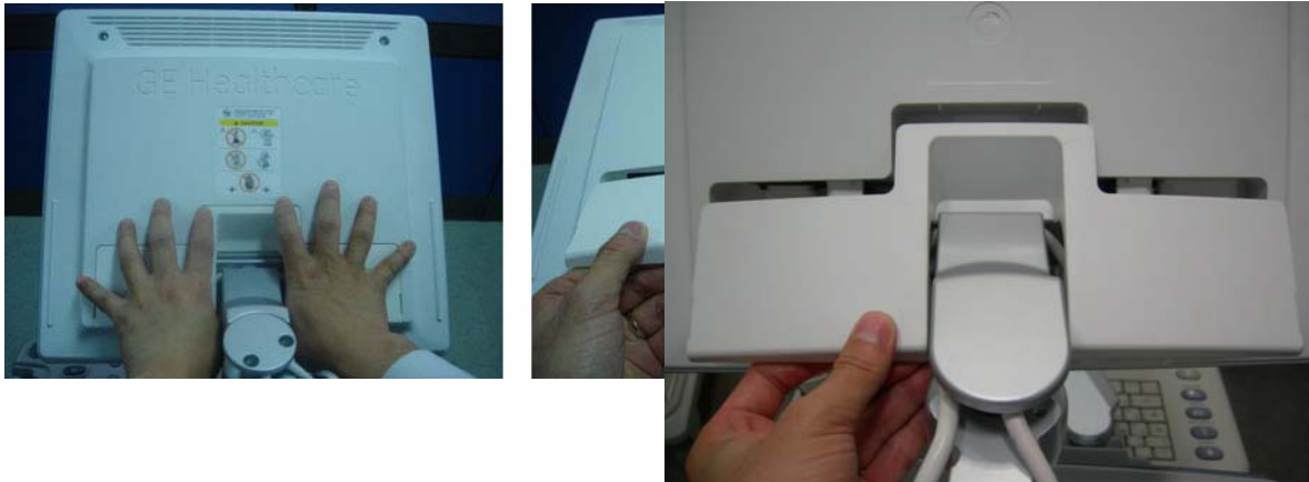
Figure 8-1 Removing the 17" LCD cable cover
