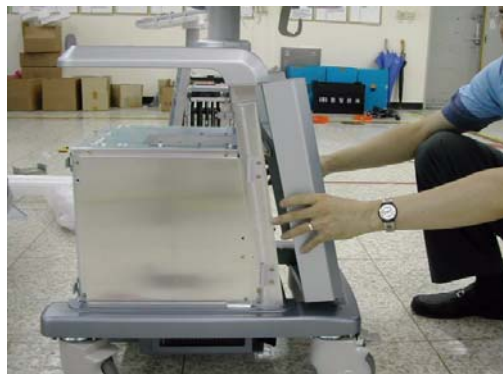
Figure 8-90 Removal of front cover
