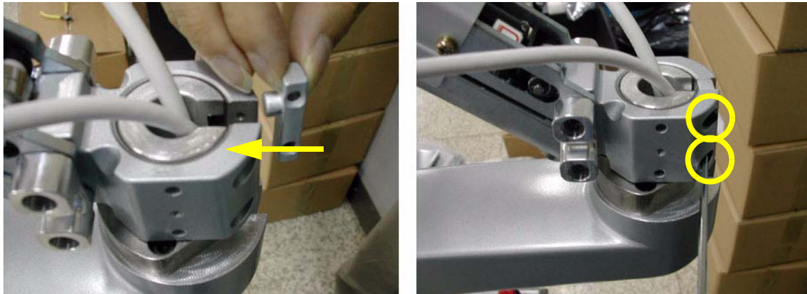
Figure 8-45 Installing the Arm stopper
