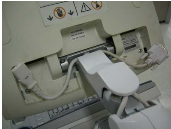
Figure 8-19 Disconnecting power cable and DVI cable
