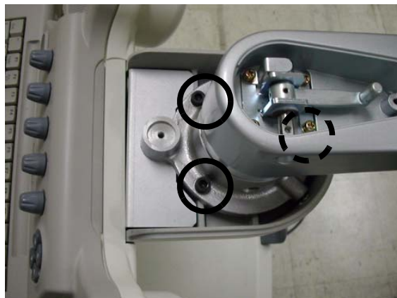
Figure 8-41 Assembling the arm neck pipe
