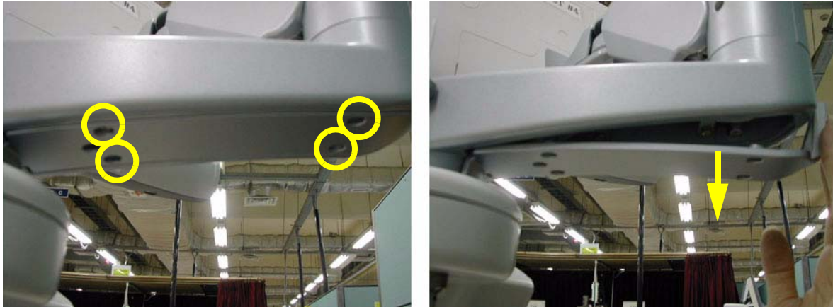
Figure 8-64 Removing the Arm bottom cover
