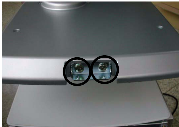
Figure 8-303 Rear Handle Installation
