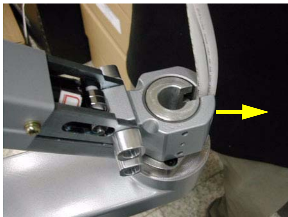
Figure 8-29 Pulling out power cable & DVI cable
