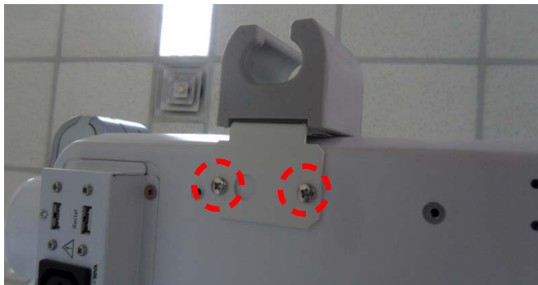
Figure 8-320 MTZ PROBE HOLDER Installation
