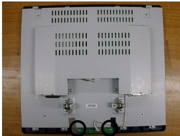
Figure 8-12 Removing the OSD Key Assy
