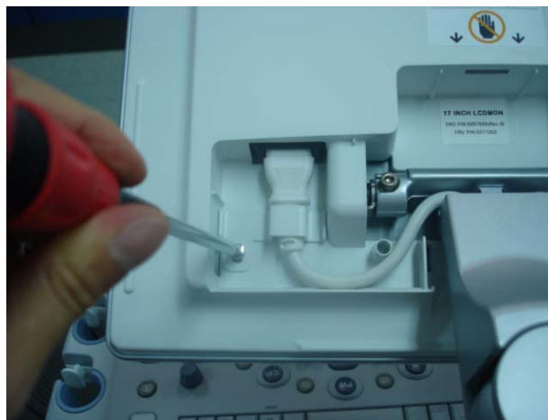
Figure 8-18 Removing the power cord bracket
