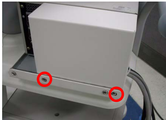
Figure 8-267 Printer VCR DVD Fixture installation top
