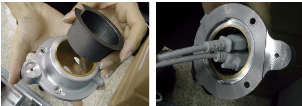
Figure 8-37 Inserting the oilless bush
