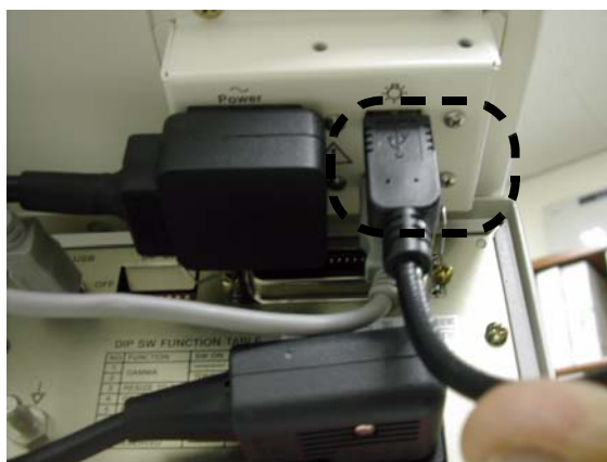
Figure 8-307 Additional Task Lamp Installation
