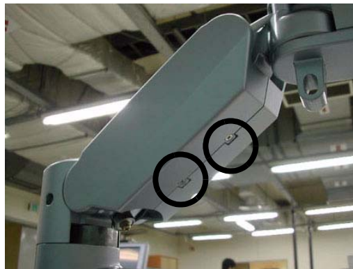
Figure 8-59 Assembling the Arm Cover L & R
