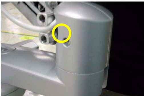
Figure 8-57 Assembling the Cam Cover L & R
