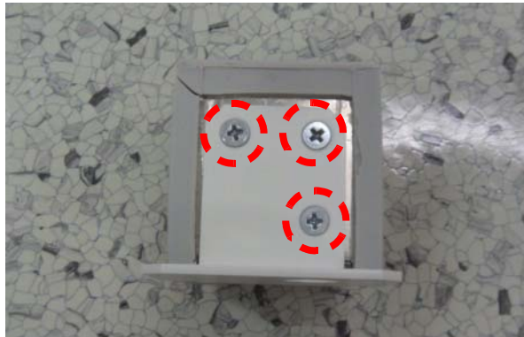
Figure 8-319 MTZ PROBE HOLDER Installation
