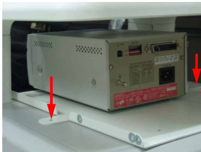
Figure 8-249 BW Printer Fixture Middle installation
