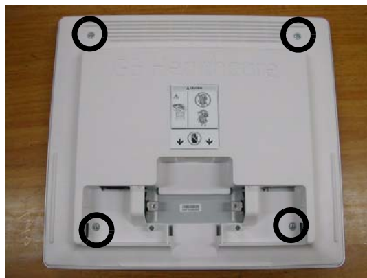
Figure 8-10 Removing the rear cover
