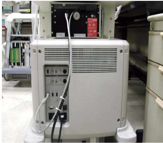
Figure 8-255 Color Printer Fixture Middle installation
