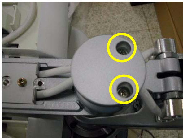
Figure 8-65 Removing the Arm cable cover
