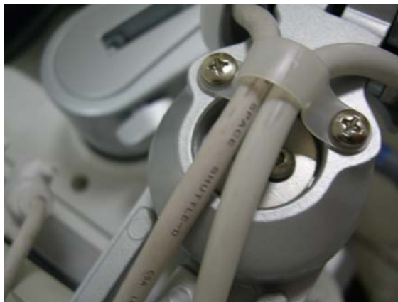
Figure 8-50 Assembling the Cable clamp
