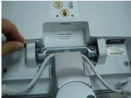
Figure 8-15 Removing the power code bracket
