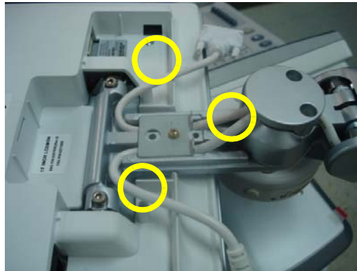
Figure 8-22 Separating the LCD monitor & Removing the Cable bracket.
