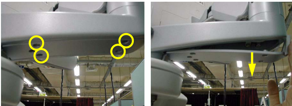
Figure 8-25 Removing the Arm bottom cover
