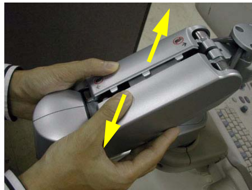
Figure 8-23 Removing the Arm cover L & Arm cover R
