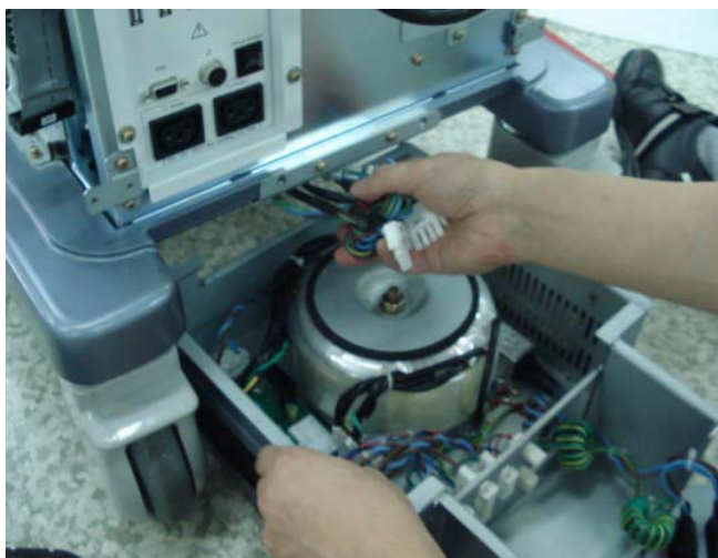
Figure 8-145 Insert the Transbox assy
