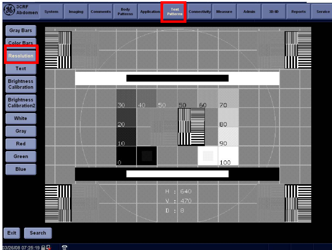
Figure 4-22 17" LCDMON II Assy Function Check
