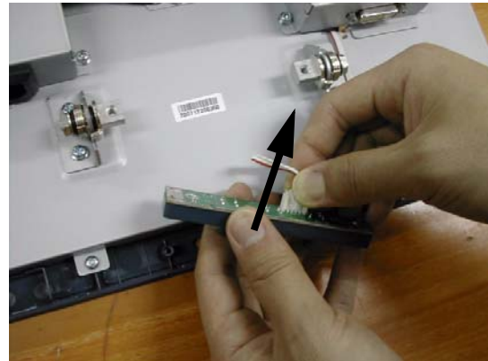
Figure 8-6 Separating the OSD key assy
