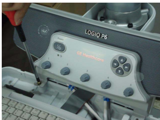
Figure 8-74 4 Screw Sub Keyboard Assy
