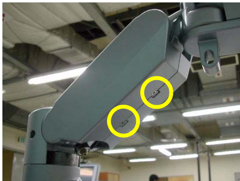
Figure 8-23 Removing the Arm cover L & Arm cover R
