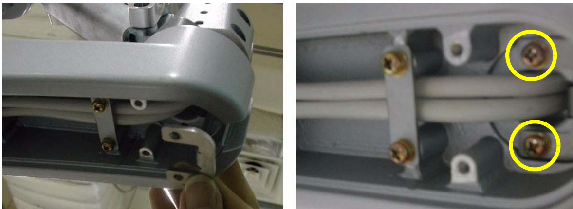
Figure 8-46 Assembling the Lower arm guide bracket
