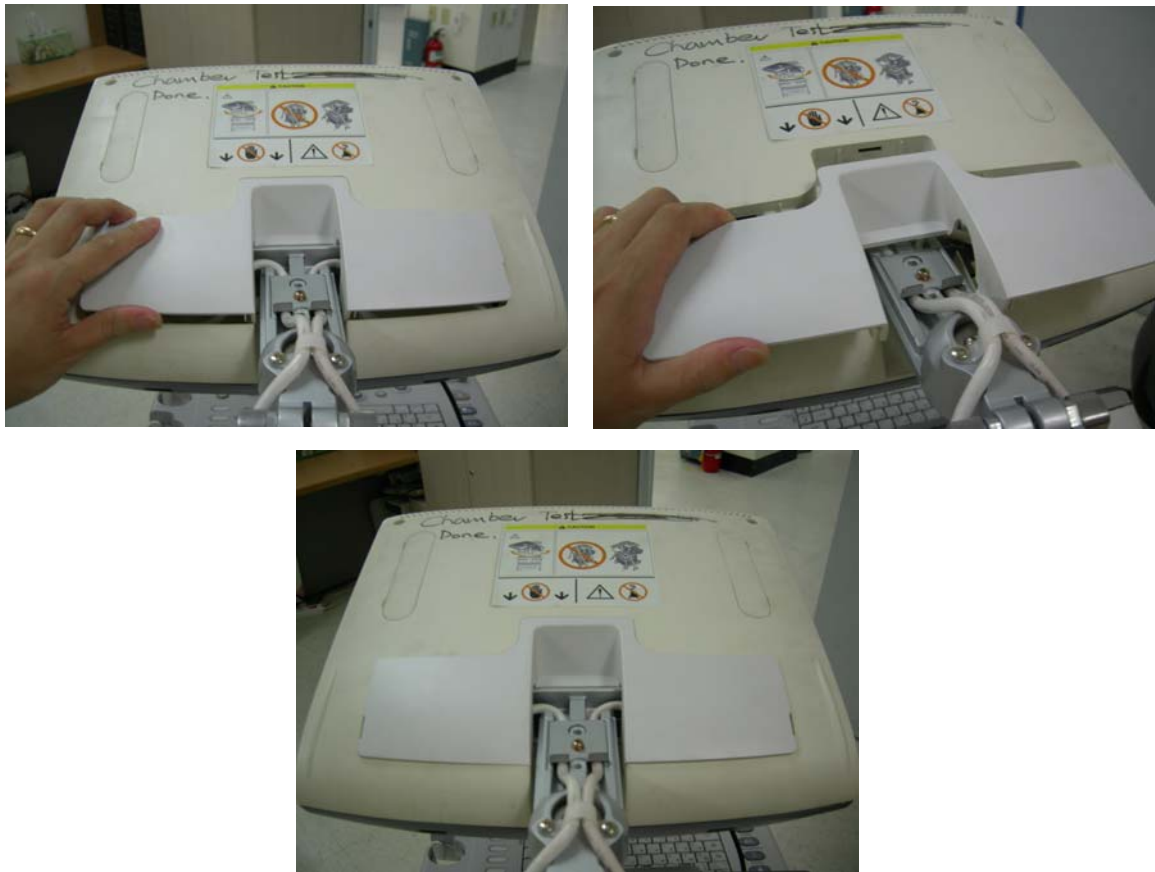
Figure 8-53 Assembling the LCD cable cover
