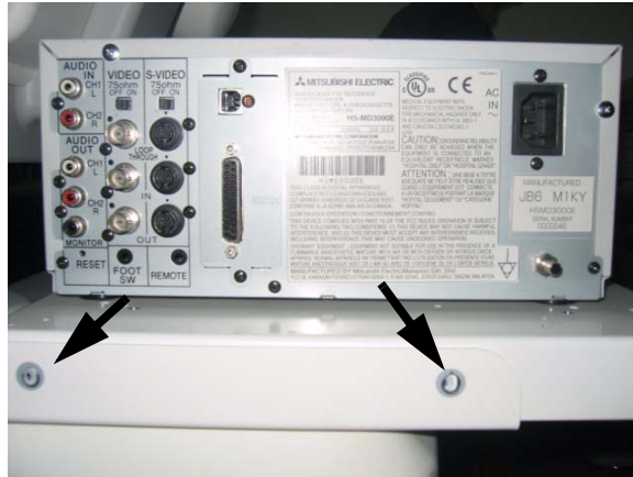
Figure 8-289 Printer VCR DVD Fixture Top installation
