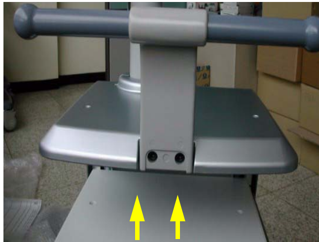
Figure 8-304 Rear Handle Installation
