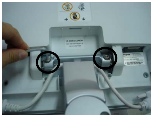
Figure 8-4 Separating the 17" LCD monitor
