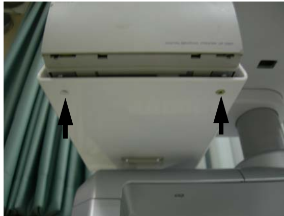
Figure 8-245 BW Printer Fixture Keyboard installation
