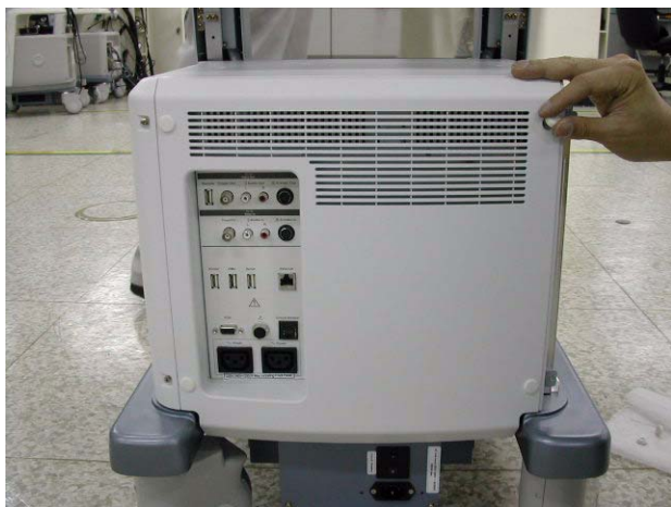
Figure 8-91 4 rubber caps and 4 screws on Rear Cover
