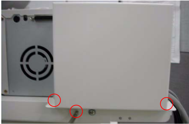
Figure 8-281 Printer VCR DVD Fixture Top installation
