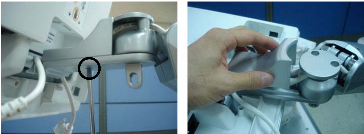
Figure 8-69 Removing the Arm fold cover
