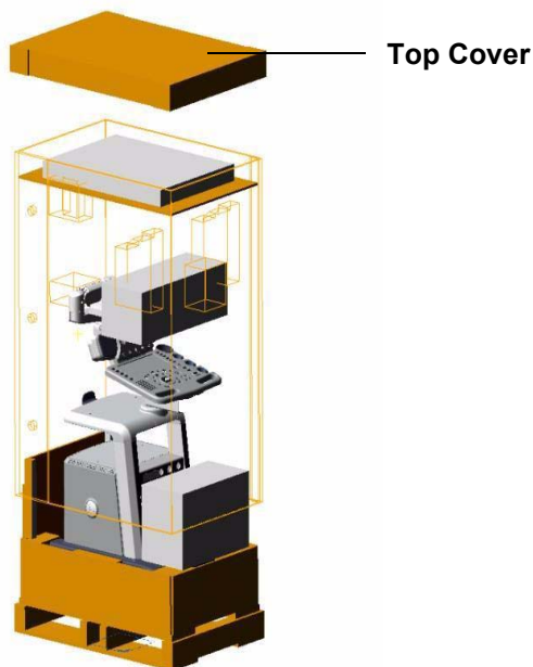
Figure 3-3 Removing the top Cover
