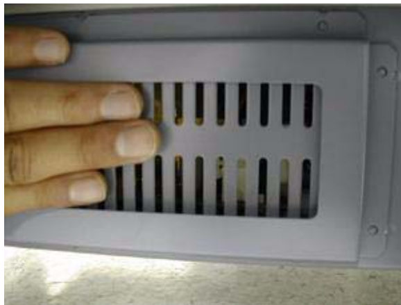
Figure 4-48 Checking Transbox fan rotating
