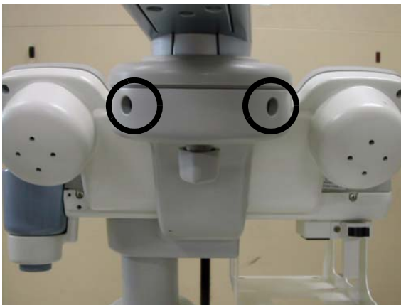
Figure 8-54 Assembling the neck front cover and the neck rear cover
