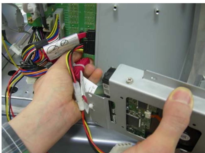
Figure 8-137 Disconnect the SATA Cable
