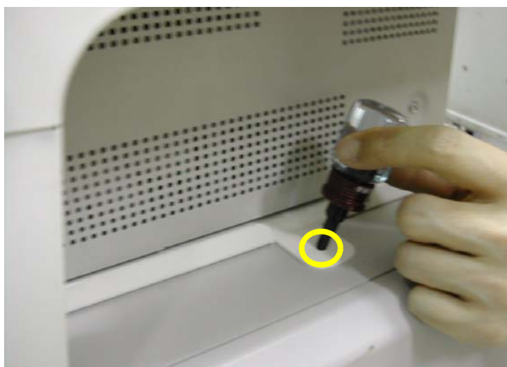
Figure 8-254 Color Printer Fixture Middle installation
