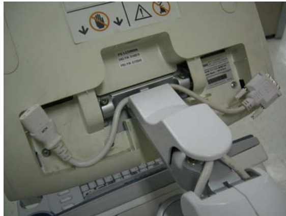
Figure 8-3 Disconnecting power cable and DVI cable
