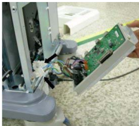
Figure 8-135 Open Rear Panel
