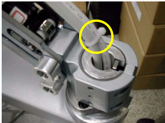
Figure 8-47 Tying the cables
