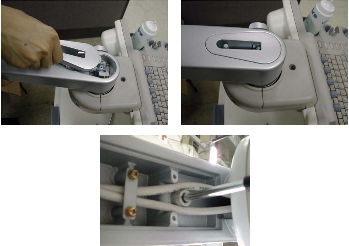
Figure 8-56 Assembling the Lock Cover
