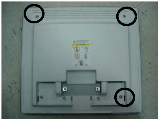
Figure 8-5 Removing the 17" LCD rear cover
