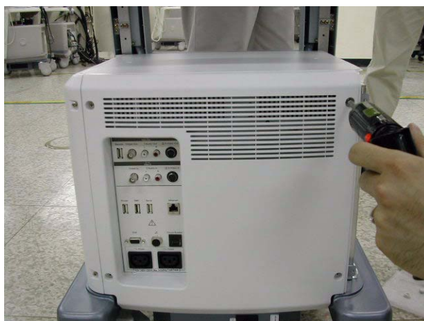
Figure 8-91 4 rubber caps and 4 screws on Rear Cover
