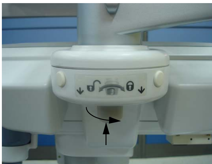
Figure 6-3 Locking the Flexible LCD arm
