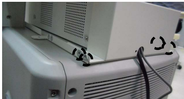
Figure 8-261 Color Printer Fixture Middle installation
