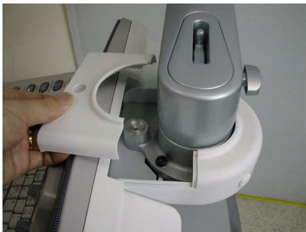
Figure 8-97 Open neck front cover
