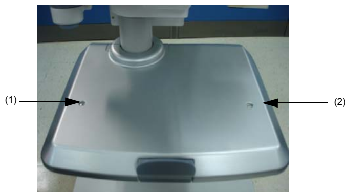
Figure 8-93 2 rubber caps of top cover
