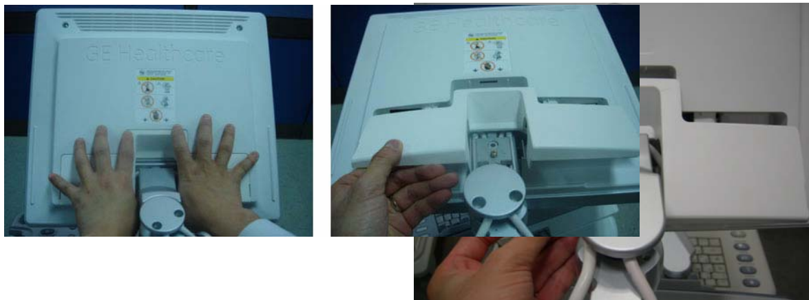
Figure 8-17 Removing the LCD cable cover
