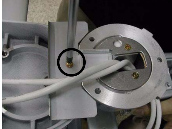
Figure 8-33 Removing OP bracket
