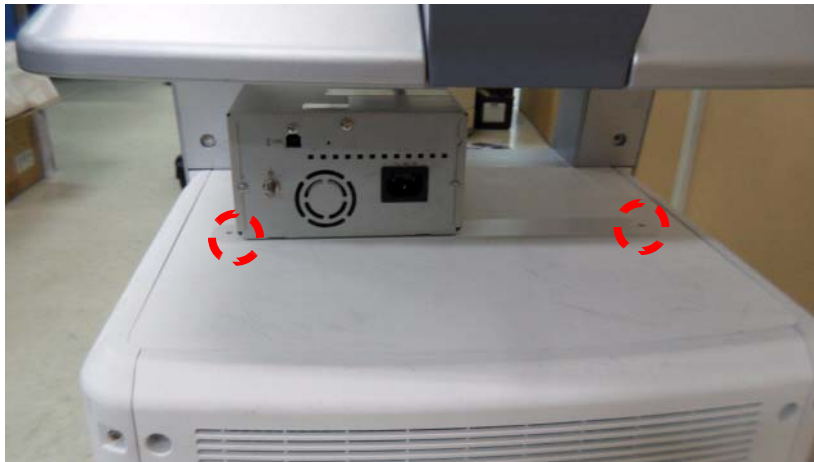
Figure 8-235 BT11 BW PRINTER Option Installation
