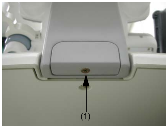
Figure 8-305 Rear Handle Installation
