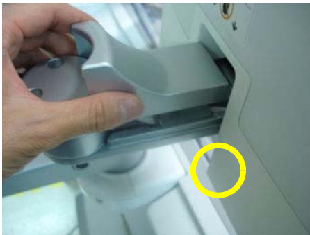
Figure 8-58 Assembling the Fold Cover
