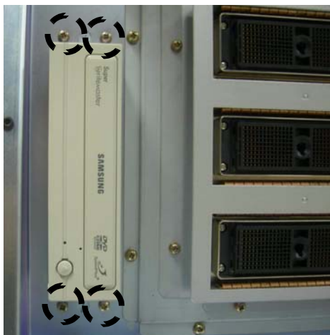
Figure 8-129 Unscrew 4screws and remove the DVD Assy
