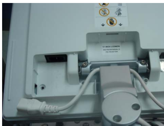
Figure 8-38 Inserting the flexible arm
