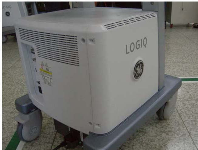
Figure 8-86 2 screw on side cover
