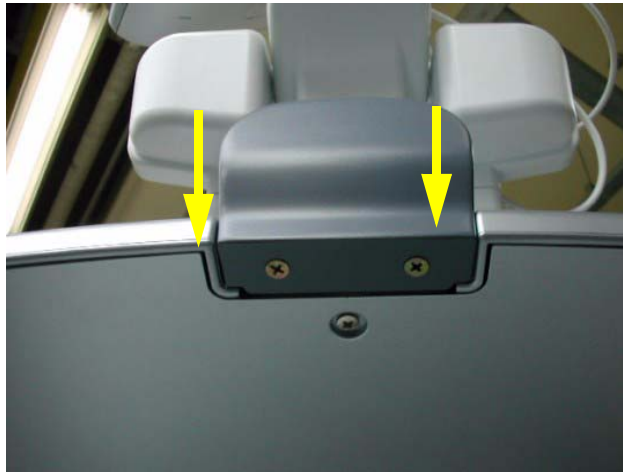
Figure 8-302 Rear Handle Installation
