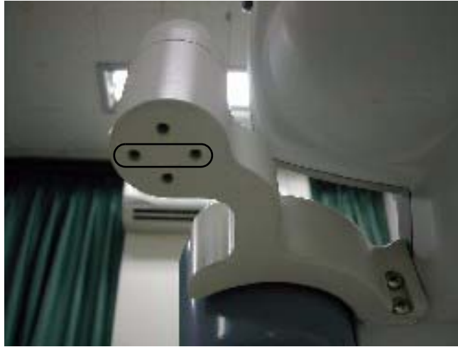
Figure 8-230 Endo Probe Holder Installation
