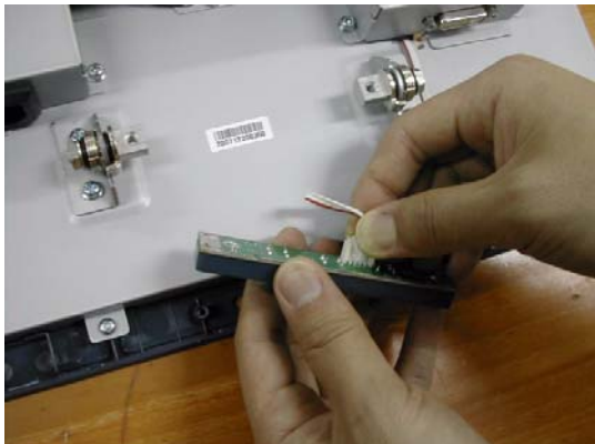
Figure 8-13 Disconnecting the cable
