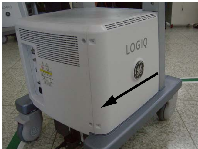
Figure 8-87 Open side cover
