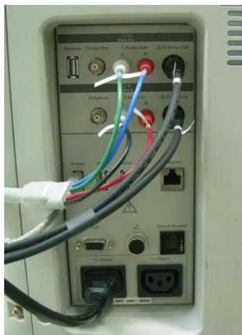
Figure 8-300 Printer VCR DVD Fixture Top installation (LQ MD800)
