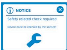
Perform an inspection according to the manufacturer's specifications every 12 months. This will be displayed on the device.
