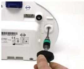
1. Loosen the screws on the back of the device by 3 turns with the recommended screwdriver (TORX - screwdriver - T10).
