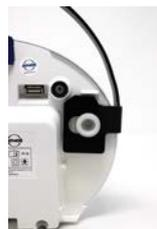
3. Insert the recesses of the carrying handle in the provided strap holder clips and press the carrying handle inwards, until it clicks into place.
