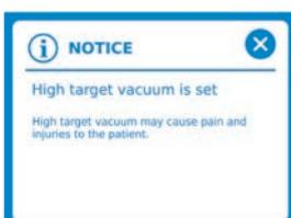
If target vacuum is adjusted over -50 mbar the notice appears „High target vacuum is set“.
