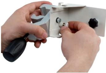
2. Turn the holder clamp until the fixing pin clicks into place at the next fixing.
