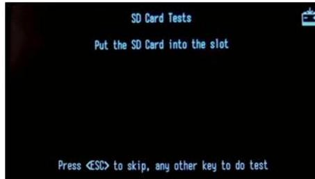
2. The SD Card Tests performs a read/write test on the SD card currently installed. The test will respond with a PASS or FAIL.
