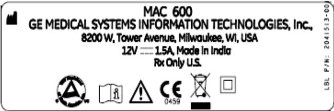
2. The new Class I product label is as follows. Place the new label on the back panel (the label is part of the 2047328-002 FRU).
