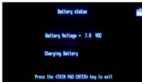
3. Check the battery voltage from this menu along with charging status.
