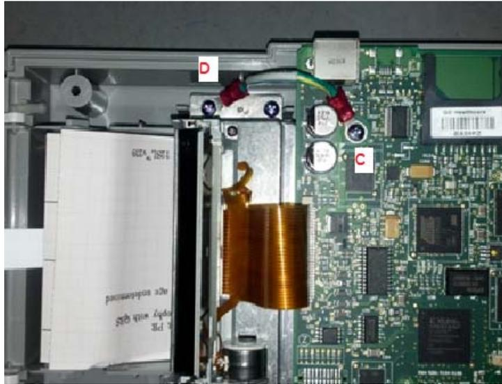
Table 4-3. Replacing the Thermal Printer
