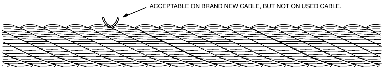
ILLUSTRATION 6 SINGLE CROWN WIRE BREAK
