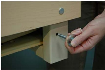
13. Fasten the bolts through the holes in both sides of the brackets and posts. This will ensure that the footboard is not accidentally removed before the footboard cord is disconnected.
