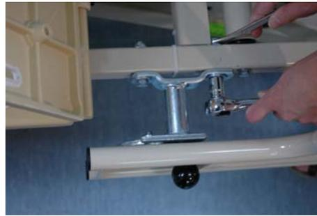
*NOTE: Raising the head deck section will allow for better access when mounting the Assist Rail™ to the bed frame.*
