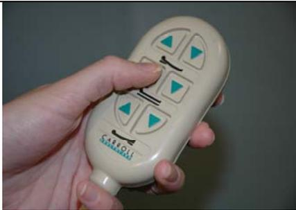
4. Remove any remaining packaging straps or material from siderails, then locate the patient hand control strapped to the side of the bed. Press the HI-LO UP button to raise bed to a comfortable working height.
