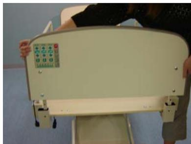
11. Place the footboard into the bracket assembly at the foot end of the bed. Ensure that the Staff Control Keypad faces out from the bed.
