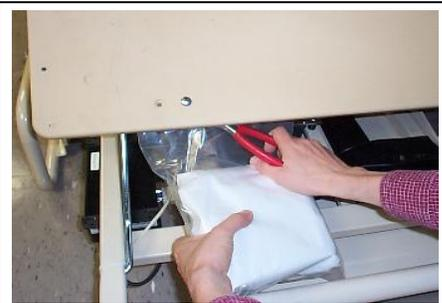
6. Lift the foot-knee deck then cut the wire tie wrap holding the mattress keeper bag, and remove. \* (If your four corner mattress keepers are already installed on each corner of the bed deck, skip to the step 8).
