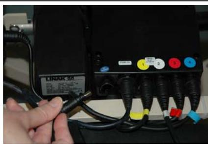
5. Raise the head section of the bed and connect the battery cable to the open port of the 120V control box. This will ensure the on-board battery remains fully charged and ready for use.
