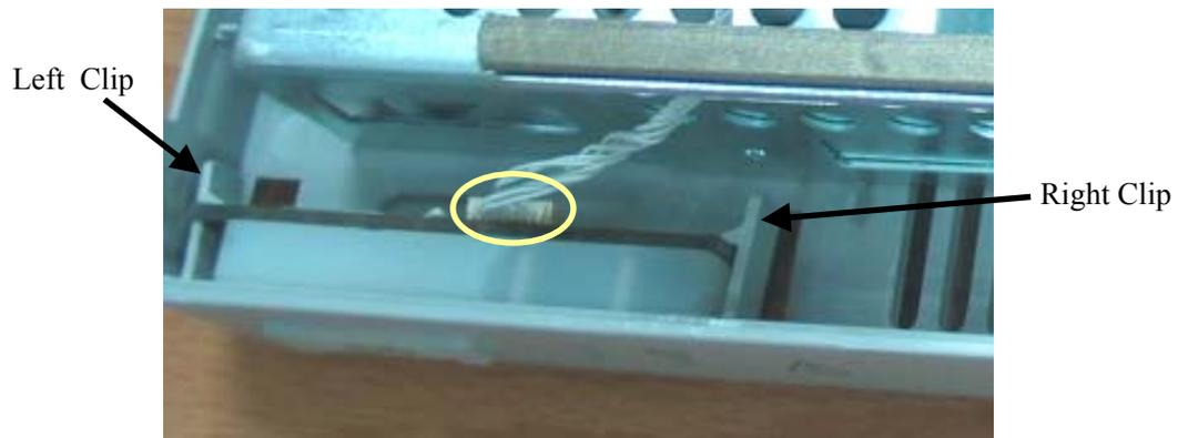
2. Release the clips with fingers. At the same time pinch the power switch & LED board, push it to the left and take it out along with the power switch.
