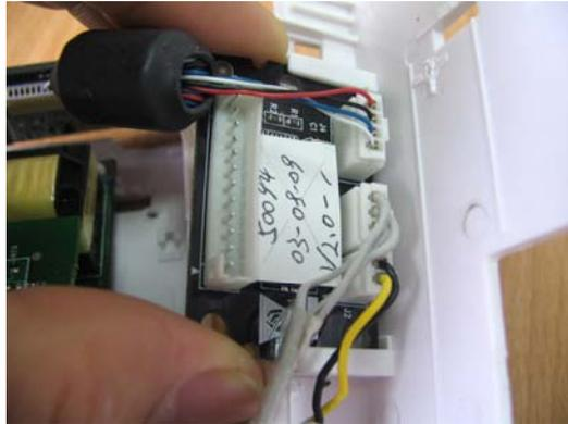
7. Take out the infrared communication board and disconnect all the cables from it.
