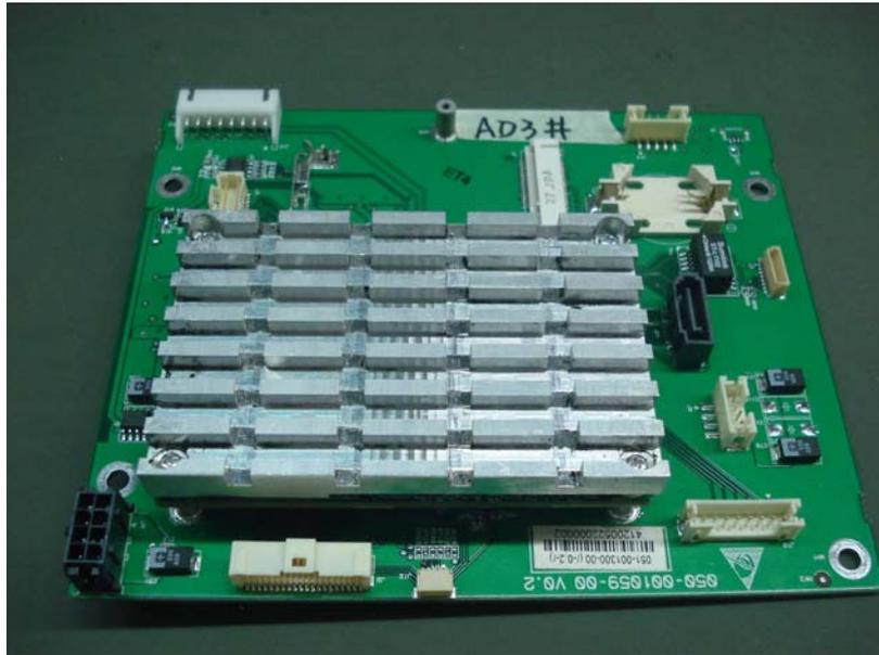
3. Unscrew the four pan head cross recessed screws and remove the cooling fin in the industrial control board.
