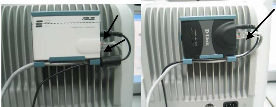
2. Press the leaf on the fix board with forceps; push the AP and installation board upwards. Then remove the AP and installation board.
