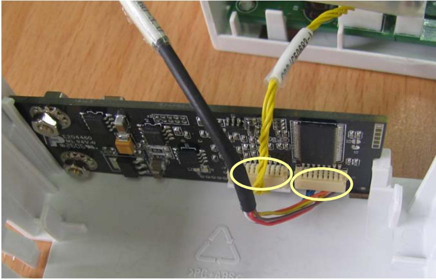
5. Disconnect the cables from the button board and unscrew the PT3×8 screw. Then release the two clips and take out the board. After that, disconnect the cable to the fan and remove the button board.
