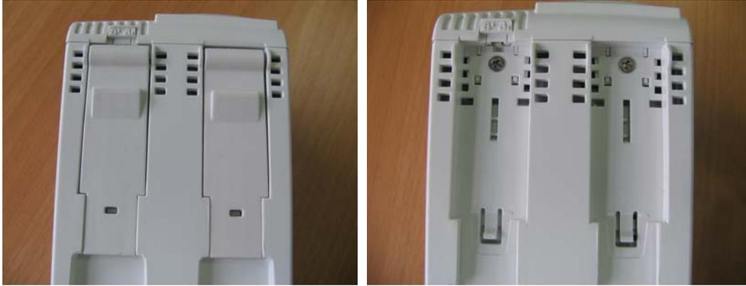
2. Take off the front cover of the CO<sub>2</sub> module by referring to the procedure as described in **5.6.1 Disassembling the ICG Module**. Then press the two clips about 1mm and take off the housing.
