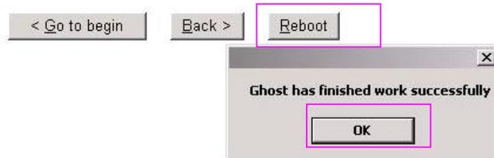
Click **[OK]**, and then click **[Reboot]**. When the monitoring screen of BeneView T8 displays, remove iView maintenance USB disk. The system will restart and enter Windows 7 system. A prompt to activate WIN7 will display.
