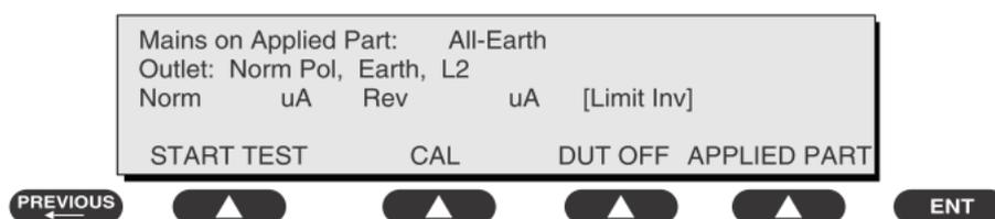
5. Select the desired outlet configuration and applied part to test using the appropriate SOFT KEYS:
