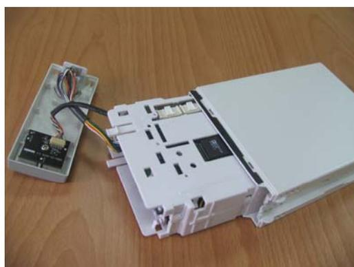
5. The side cover of the module without the housing is composed of two halves. Release the three snaps to separate the two halves.
