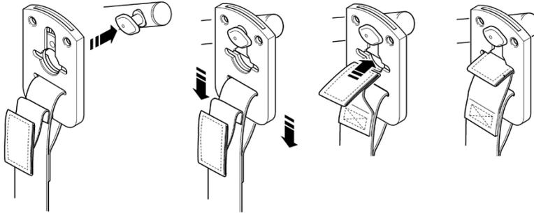
Securi3 sling attachment system. Example of installation.
