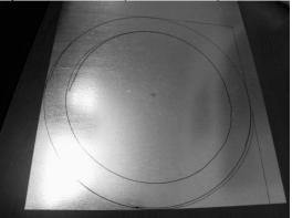
3. Use metal shears to cut out your design from the sheet metal. You may need to bend the metal up or down as you cut.
