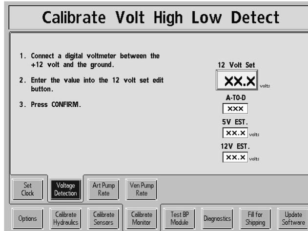
1. Open the monitor unit and connect a Digital Voltmeter between the +12 volt test and the ground test points shown in Figure 7.
