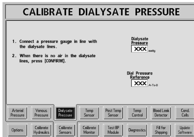
2. Dialysate should be flowing, as indicated by the flow indicator in the dialysate lines.
