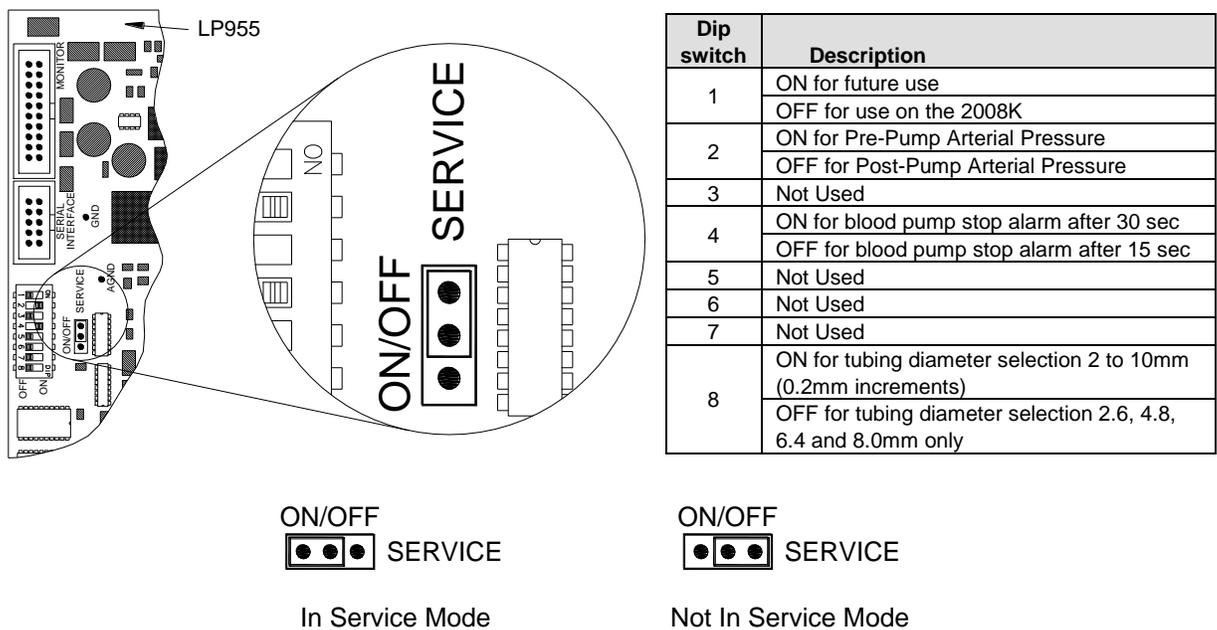
**Figure 5 - Blood Pump DIP switches & Service Jumper**
