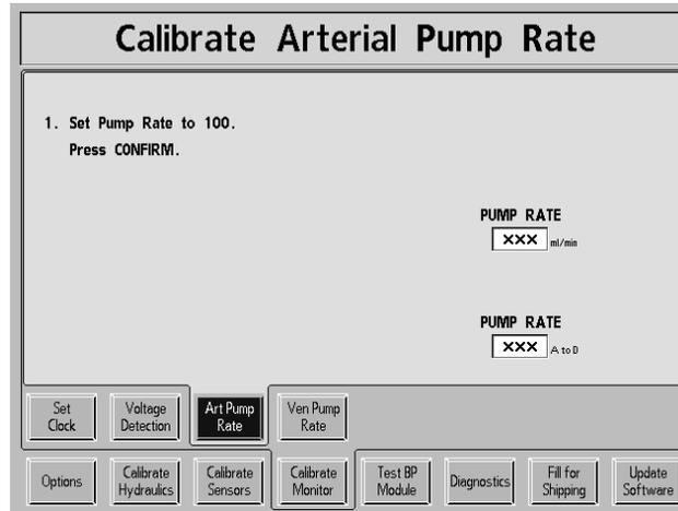
1. Adjust the arterial pump rate to 100ml/min.
