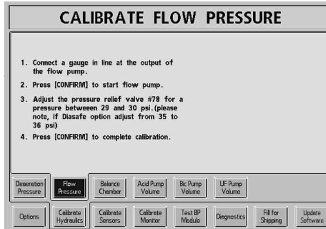
1. Connect a gauge in line at the output of the flow pump (See Figure 1, pg. 5).
