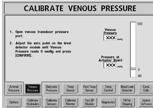
1. Open the venous transducer port  $P_{VEN}$  on the level detector module to air (atmospheric pressure).
