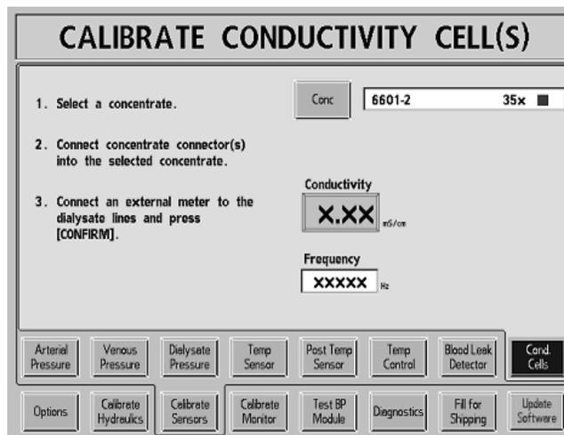
1. Identify the concentrate you will be using to calibrate the conductivity cells.
