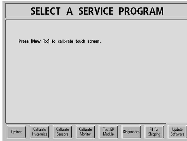
Select a calibration by touching the appropriate calibration button. A second row of buttons will appear above the first.
