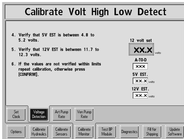
4. Verify that the 5V EST. displayed on the screen is between 4.8 and 5.2 volts.
