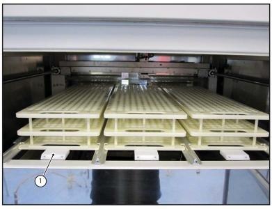
Figure 1.5 3060-tube (high-speed) Stockyard Latching Mechanism
