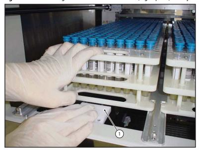
Figure 2.16 Removing a Rack from the 5440-tube (high-speed) Stockyard
