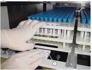
Figure 2.14 Removing a Rack from the 3060-tube (high-speed) Stockyard
