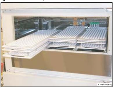
Figure 2.12 A Rack Not Fully Removed from a Shelf Unit of a 3060-tube Stockyard
