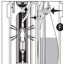
**CAUTION:** Ensure all four cassette latches are clearly visible after the cassette is installed. Refer to *Loading the Cassette* on page 35.
