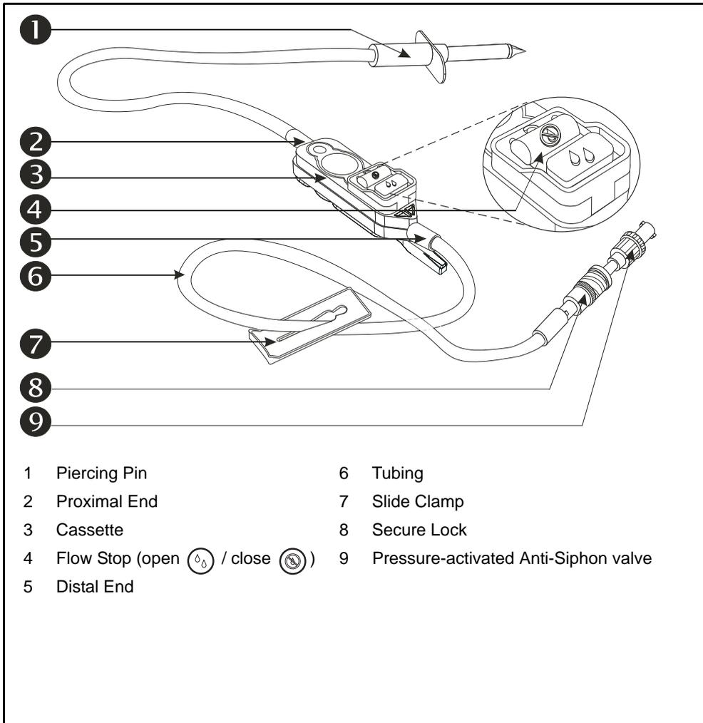
**WARNING:** ALWAYS prime the pump set to remove air from the cassette, tubing, and injection sites prior to connecting to the patient. ALWAYS disconnect the pump set from the patient prior to priming or purging. Arrange tubing, cords, and cables to minimize the risk of patient strangulation or entanglement.
