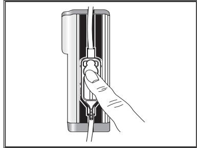
**CAUTION:** Ensure all four cassette latches are clearly visible after the cassette is installed. Refer to *Loading the Cassette* on page 35.
