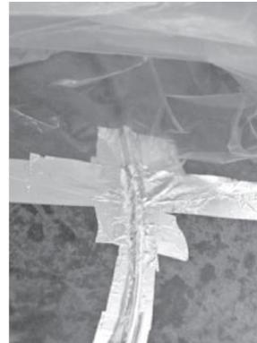
6. Put the bottom part of the decontamination bag on top of the aluminum tape, and then seal it with another layer of aluminum tape. Use multiple layer of aluminum tape (*at least 2 layers*) on both directions to ensure leak tightness.
