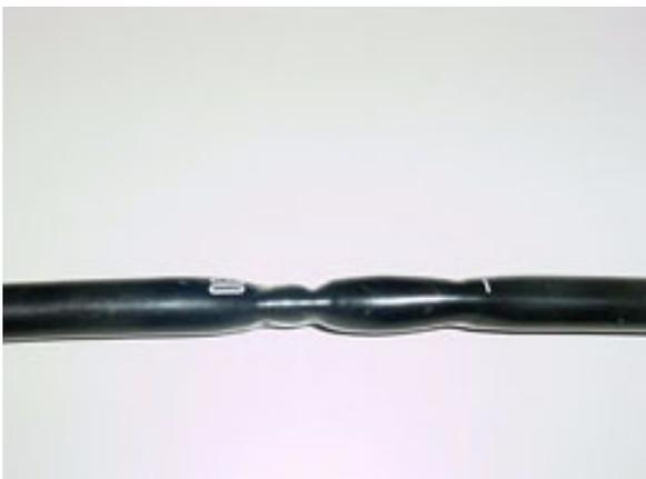
**Bite marks on transducer shaft.**
