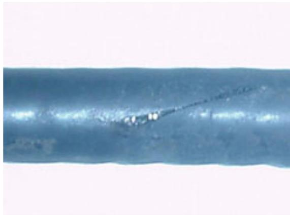
**Slice on the outer sheath caused by a scalpel.**
