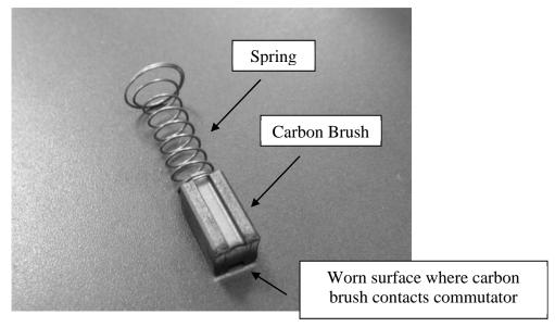
Carbon brushes slide into brass guide sleeves on opposite sides of the commutator. The brass guide sleeves align the carbon brushes with the motor.
