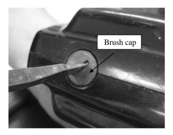
Check the carbon brushes if the motor does not start. Carbon brushes that are too short to provide full contact with the commutator must be replaced or shimmed.
