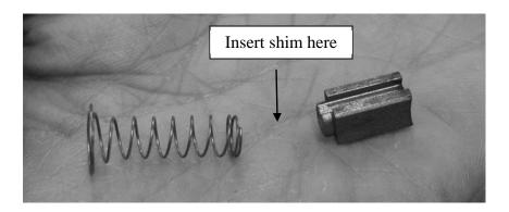
Shims may also be placed between the spring and the brush cap. The spring will be held in place in both positions by the force of the spring.
