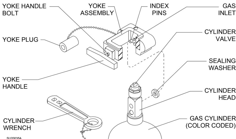
3. Insert the head of a gas cylinder with matching gas into the yoke from below, so that the gas outlet and indexing holes on the cylinder head are facing the gas inlet and indexing pins on the yoke assembly.
