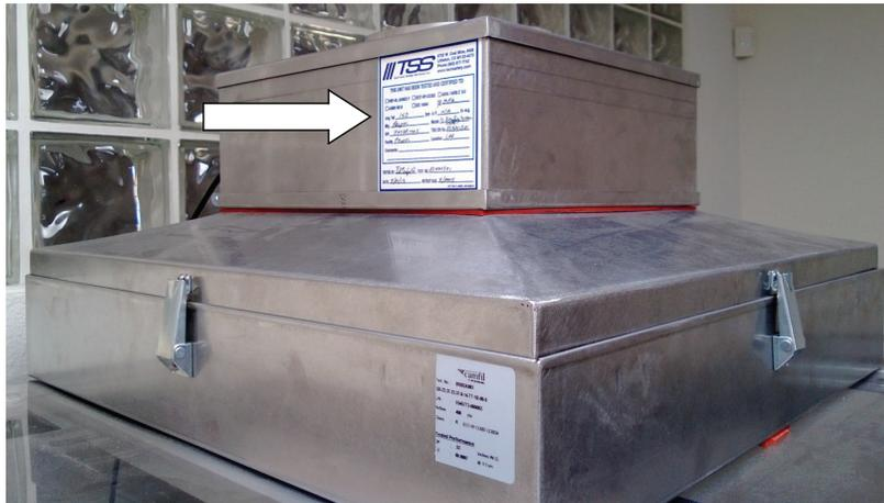
Fig. 13. Apply the onsite certification certificate onto the air generator.
