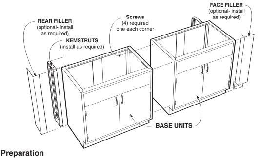
Locate and mark hood and base cabinet locations making sure area is clear of obstructions and debris. Be sure all conduit, duct work and service lines have been run and are ready for final connections.
