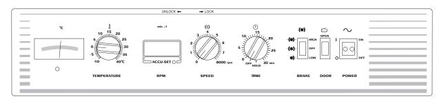
Figure 1-4. The Control Panel (Refrigerated Models)
