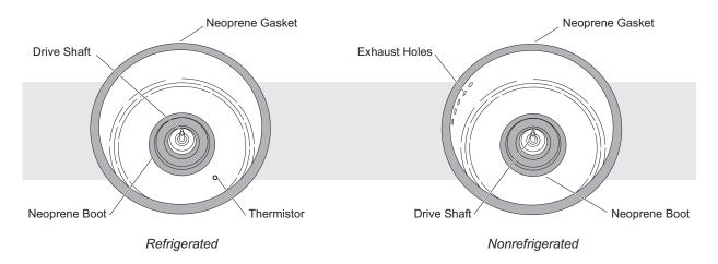
Figure 1-2. Interior View of the Centrifuge
