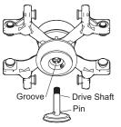
6. Load the rotor according to the rotor manual. Always run the rotor with a balanced load; fill all positions on a swinging bucket rotor yoke with buckets and/or carriers.
