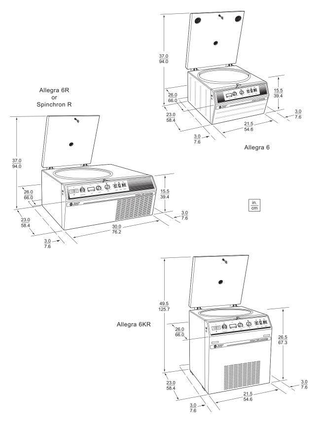
Figure 2-1. Centrifuge Dimensions
