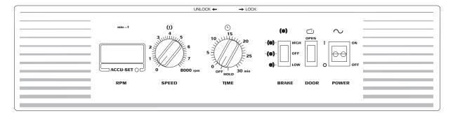
Figure 1-3. The Control Panel (Nonrefrigerated Model)
