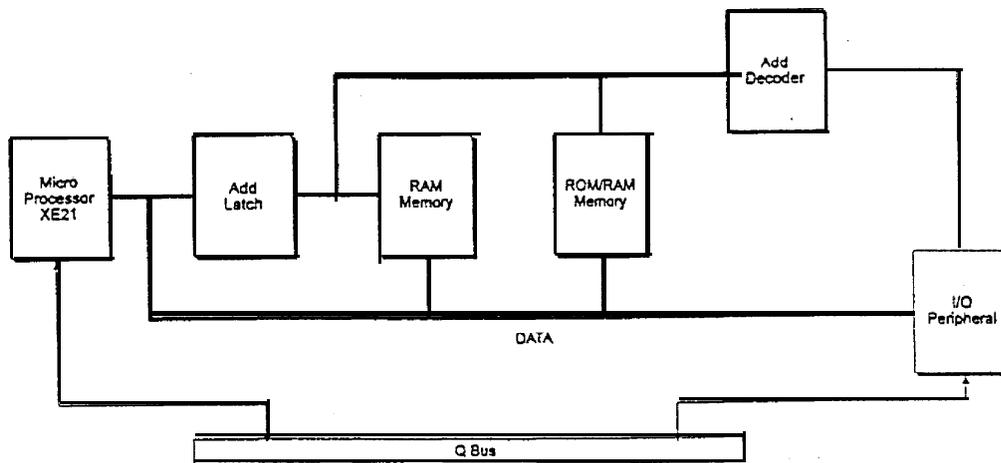
Figure 2-11: CPU Block Diagram
