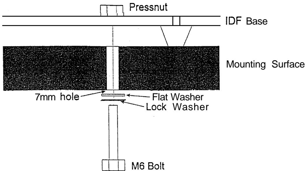
Figure 3-1 IDF Anti-Seismic Clamp
