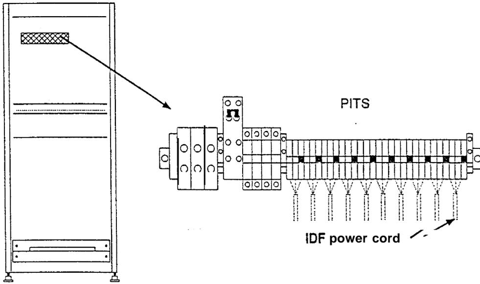
Figure 3-2 DLX1 | DLX2 Cabinet with PITS Detail
