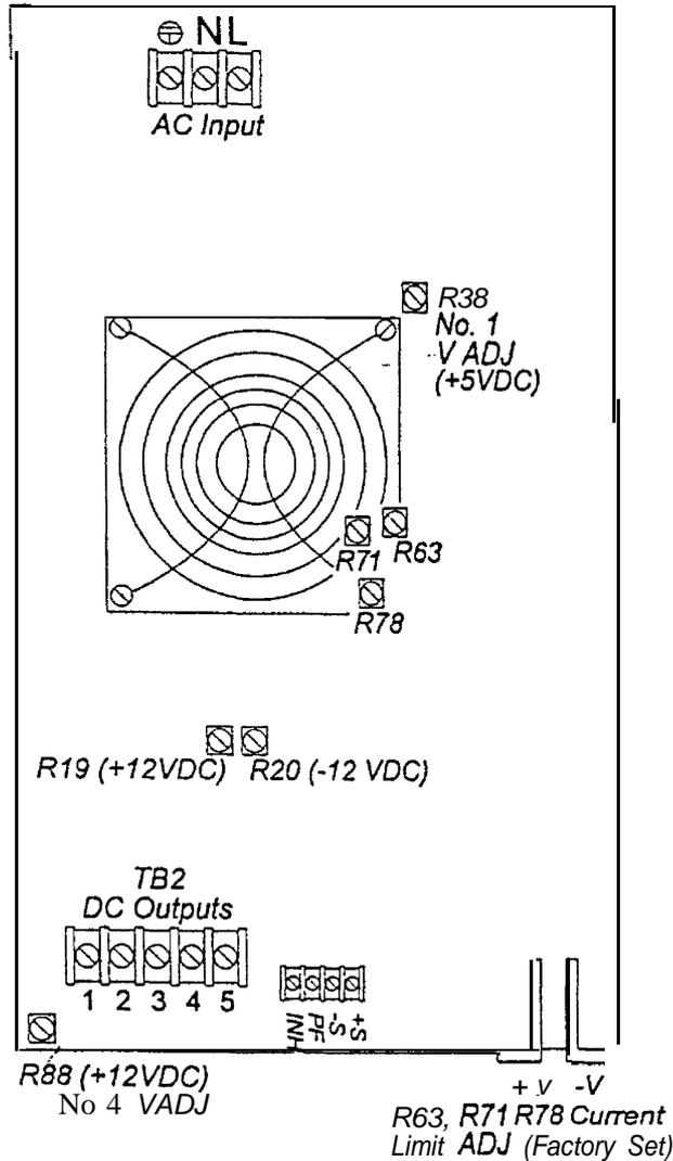
Figure 5-1: Power Supply Layout
