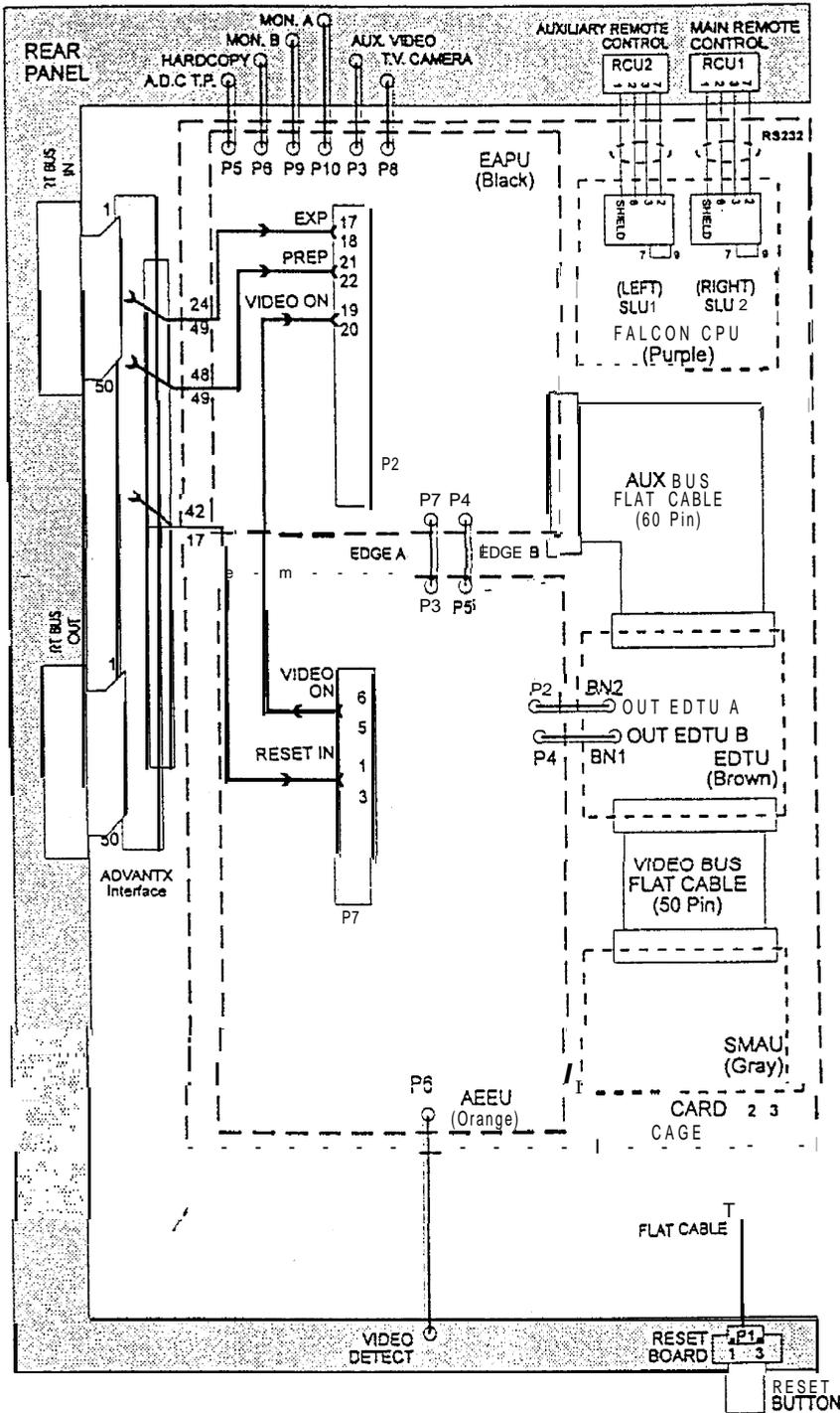
Figure 2-3: Internal Cable Interconnection Diagram
