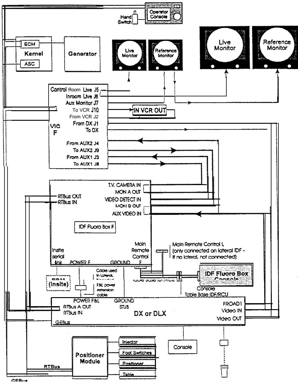
Figure 3-4 IDF Cabling Diagram
