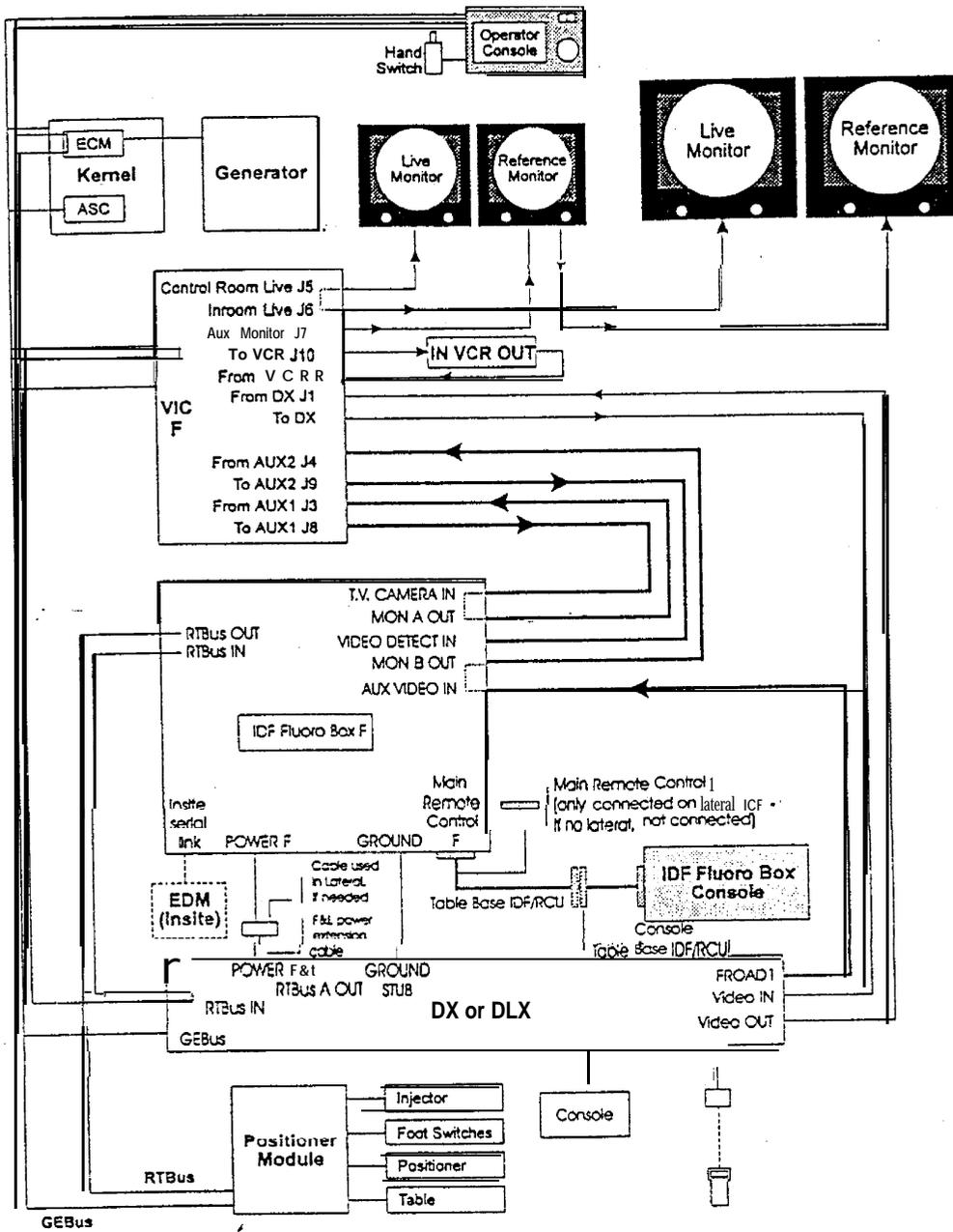
Figure I-1: IDF Image Processing System
