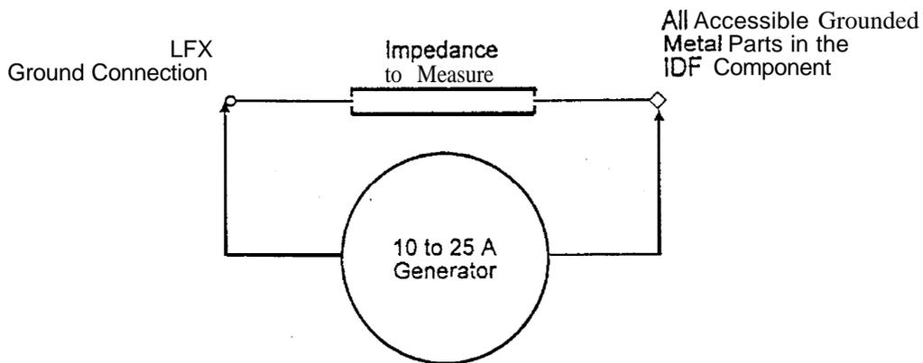
Figure 3-6: Installation Ground Cables Check Procedure
