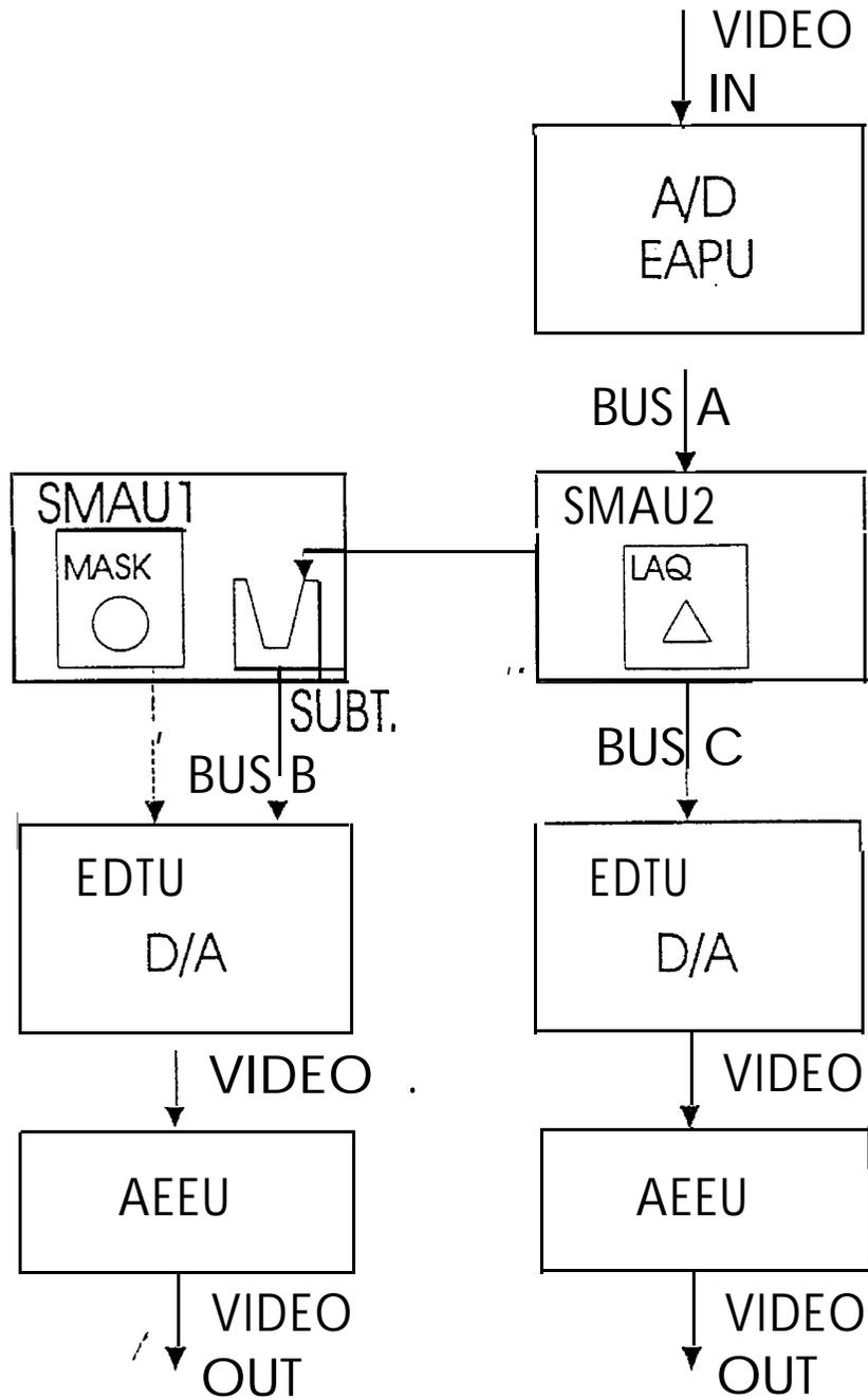
Figure 2-13: Subtracted Acquisition Software Flowchart
