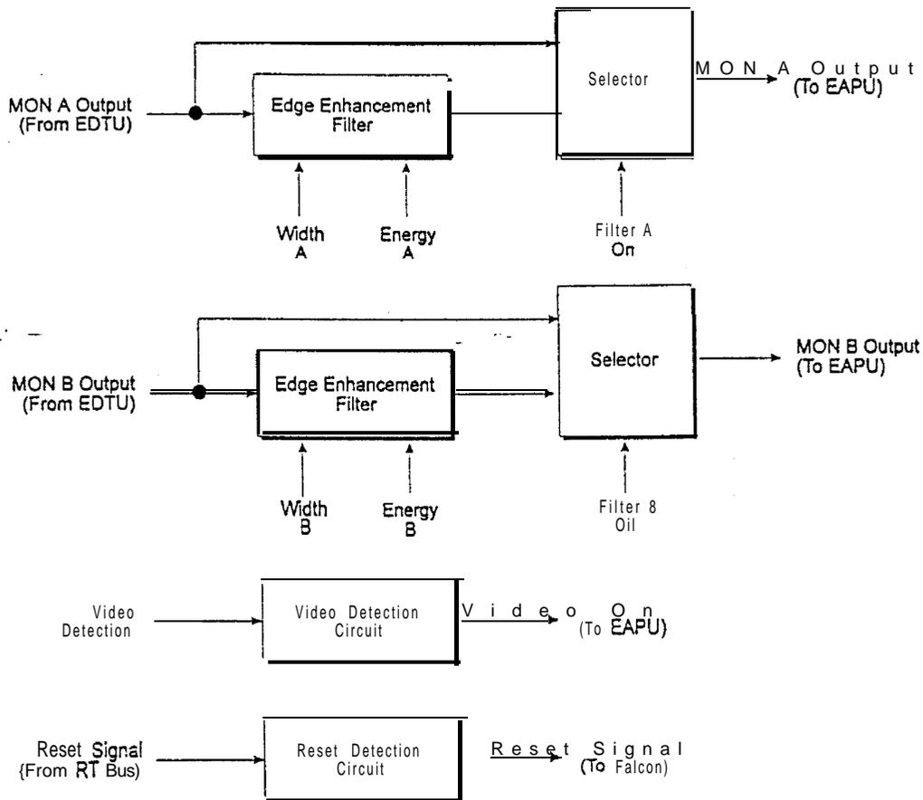
Figure 2-10: AEEU Block Diagram
