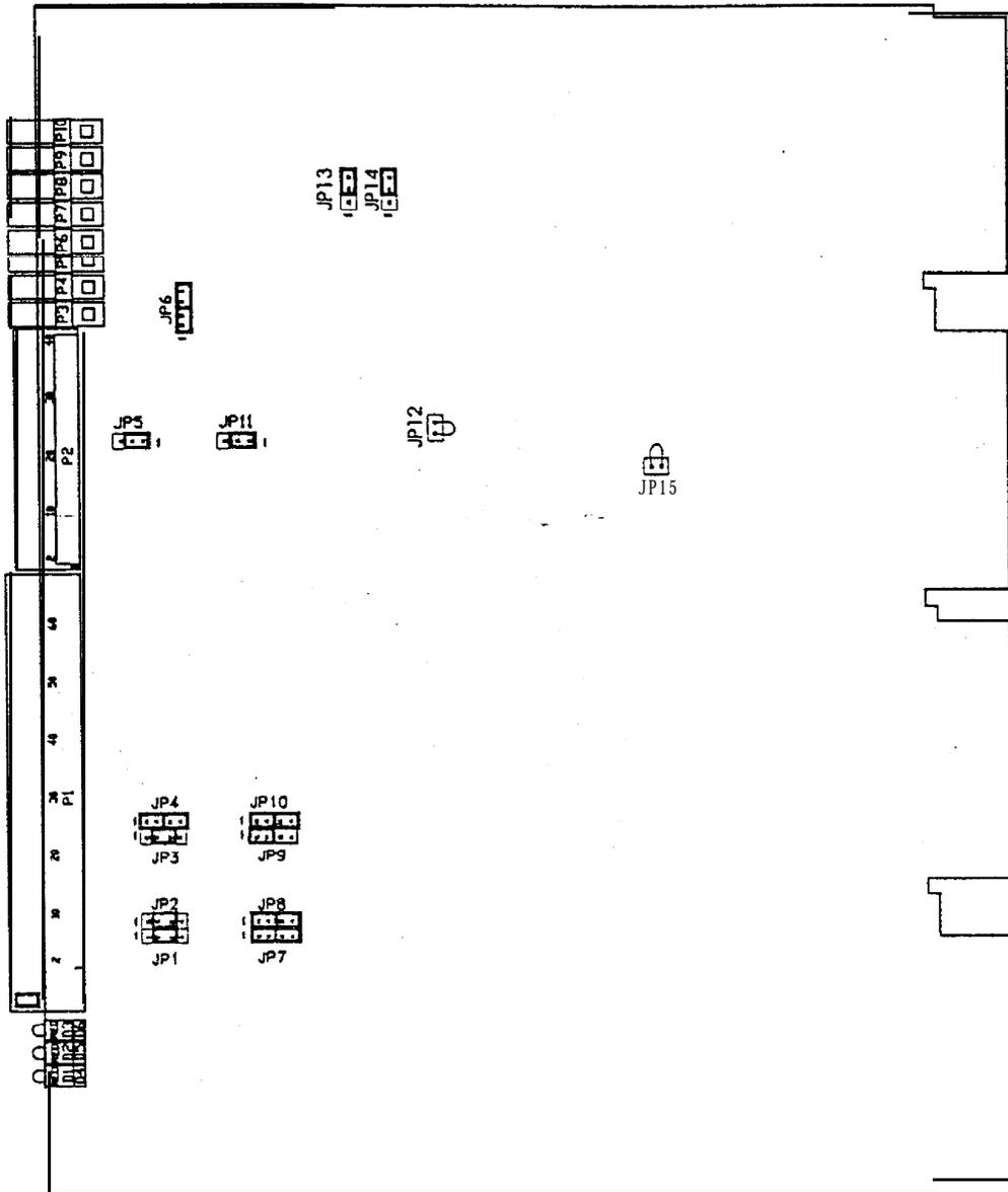
Figure 3-8: EAPU Board Layout Diagram
