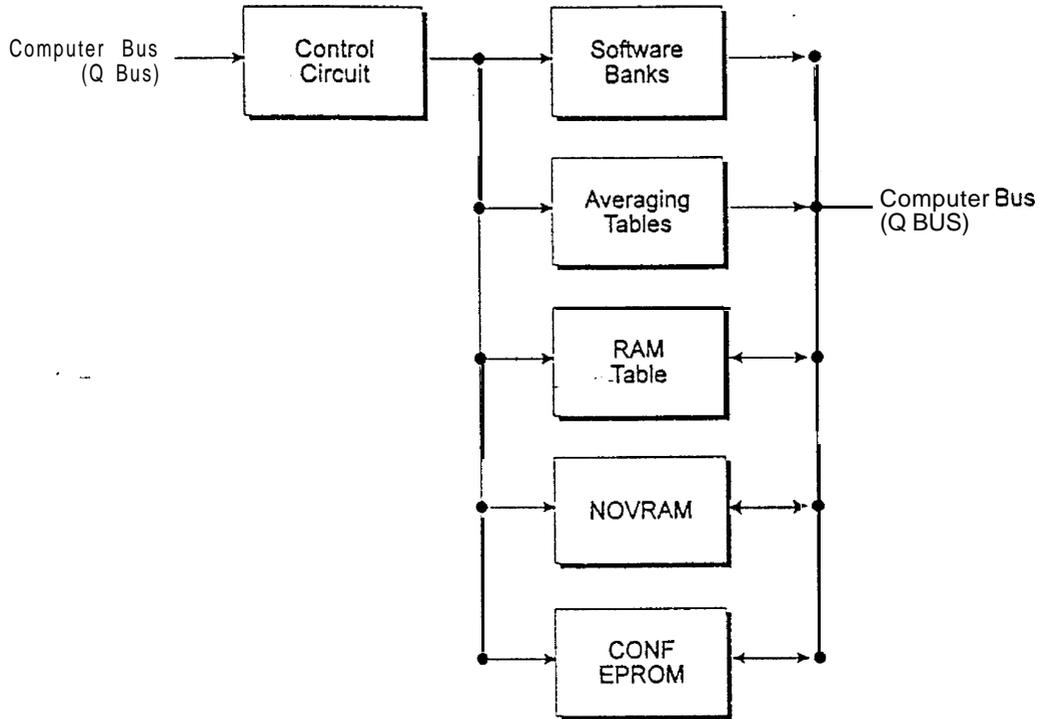
Figure 2-6: ETBM Block Diagram
