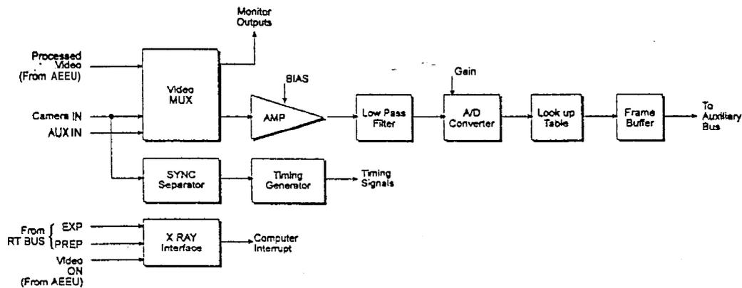
Figure 2-7: EAPU Block Diagram
