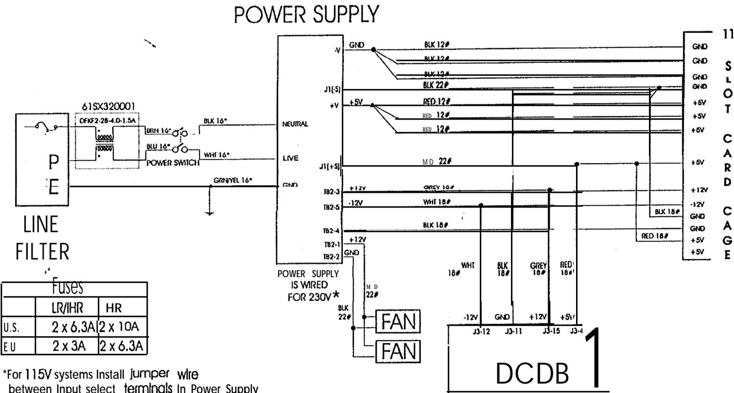
Figure 3-12: Power Connections Schematic
