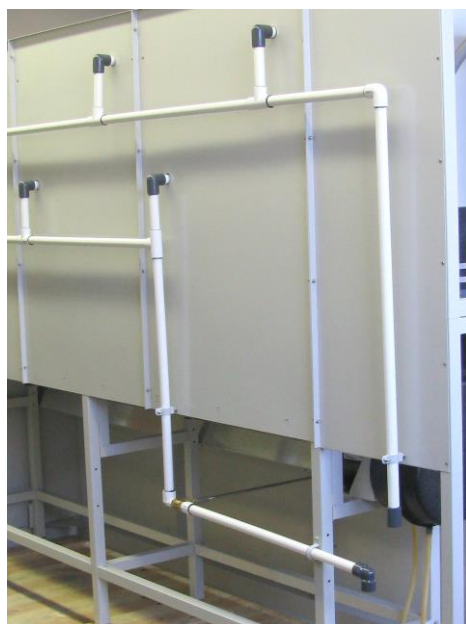
Distillation Manifold Tap Water Connections Figure 2-3
