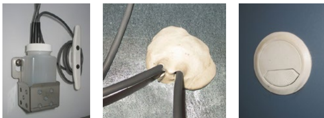
Left: Probe bottle with temperature and chart recorder probes. Middle: Top access port. Right: Side access port.
