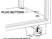
ADJUSTMENT BOLT (accessible thru cabinet bottom with straight blade screw driver)
