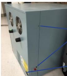
Phillips screws to remove back panel (2 on each side)
