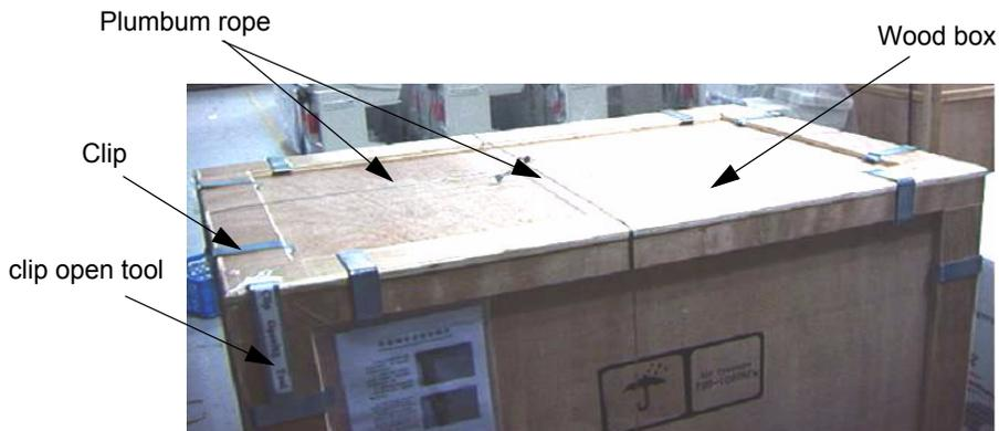
Figure 3-8 Unpacking procedure (1)
