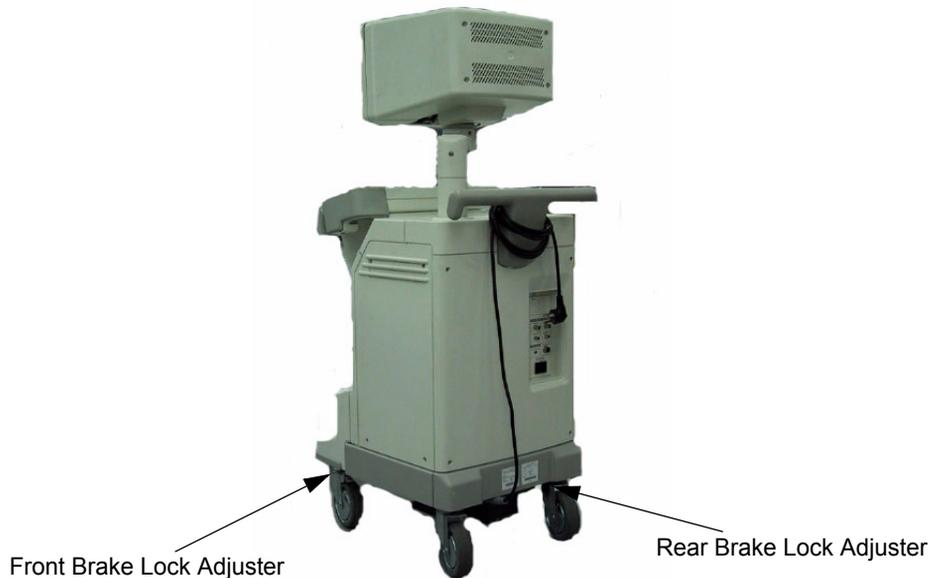
**Figure 6-38** Locations of Brake Lock Adjusters
