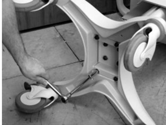
2. Remove the remaining bolts and mounting plate.
