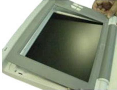
3. Remove the ten screws that secure the assembly to the display cover.
