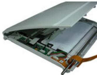
5. Disconnect all the cables from the LVDS board on the display assembly.
