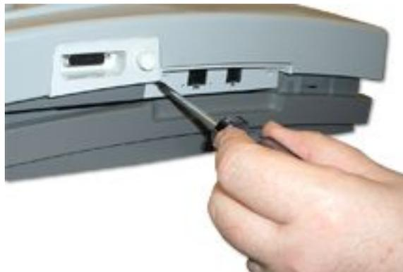
3. Grasp the side edges of the communications board and work it back and forth in the slot as you pull it out along its rails.
