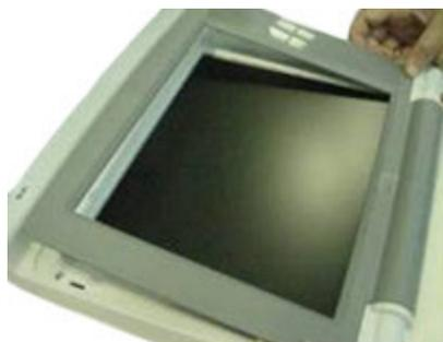
10. Reattach the display assembly to the device.
