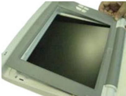
14. Reattach the display assembly to the device.
