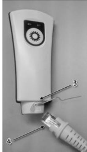
4. Insert the new cable into the handle of the barcode reader until it snaps into place.
