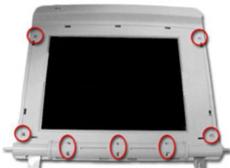
4. Gently flip over the display assembly, so the LCD panel is face down, and remove the display cover.
