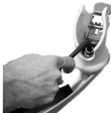
6. Install the wheel and attach it with the wheel bearing shaft and nut.
