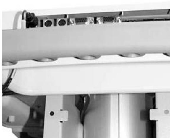
4. At the front, hold the cable to the side so it clears the front panel as you replace the panel.
