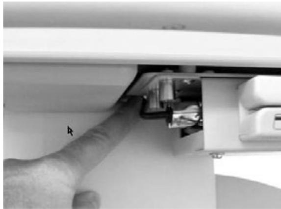
5. Plug the cable connector into port A then replace the back panel.
