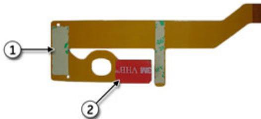
These stickers will need to be peeled in step e and step f to expose the adhesive used to affix the flex cable to the display bezel.
