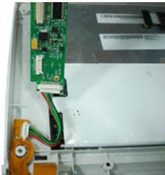
9. Position the LVDS board as shown and firmly press until the adhesive pads firmly adhere to the display bezel.
