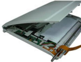
12. Gently flip over the assembly so the LCD is facing up and reattach the ten screws that secure the assembly to the display cover.
