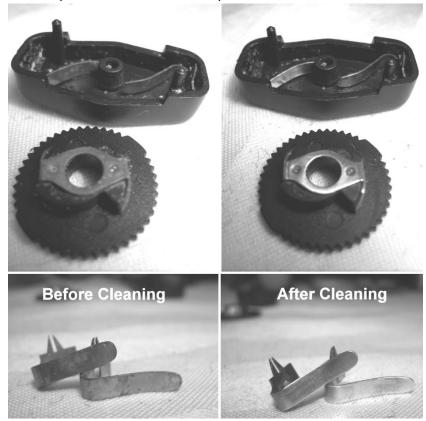
Here is a picture of the blades from a toggle switch before cleaning (left) and after cleaning (right).
