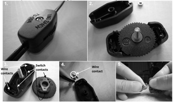
Here are pictures of the cleaning procedure with a toggle switch
