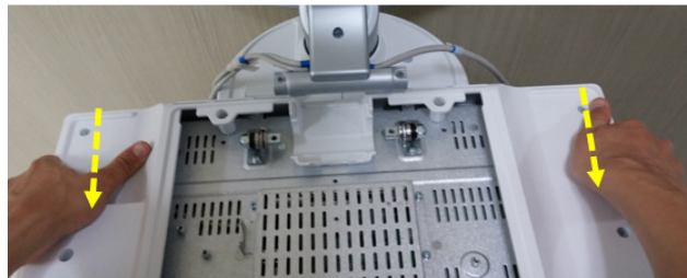
Figure 8-63 Unscrewing 2 screws & separating the Monitor
