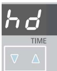
2. During continuous operation, the centrifuge will continue running until you stop it manually with the
