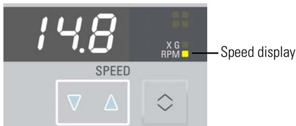
2. When the upper indicator is lit the display shows the RCF value. Press the
