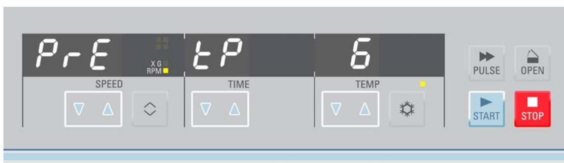
2. Enter the desired value by pressing the key
