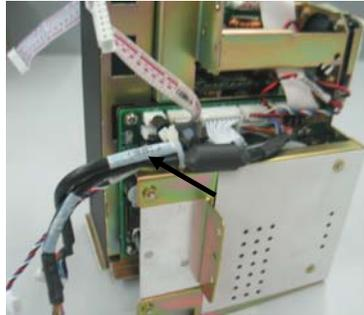
2. Unscrew the three M3×6 crosshead screws with a screwdriver and take out the NIBP rack.
