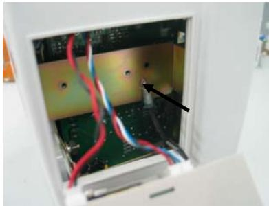
3. Unscrew the five M3×6 crosshead screws with a screwdriver and take out the main rack assembly.
