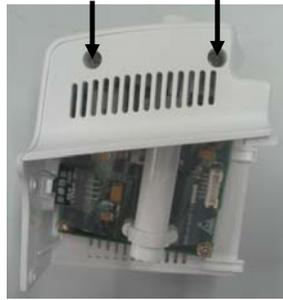
3. Unscrew the four M3×6 crosshead screws with a screwdriver and remove the Temp module main board.
