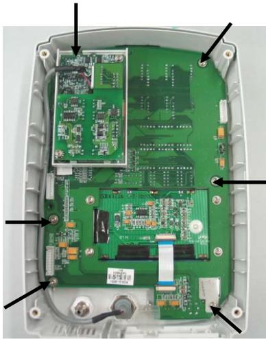
2. Unscrew the four M3×8 crosshead screws with a screwdriver; disconnect the flexible cables on the button board; and then remove the LCD.
