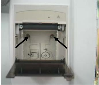
2. Remove the cables from the recorder and unscrew the M3×6 crosshead screw with a screw driver.
