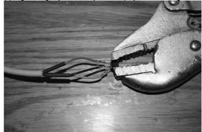
7. One at a time, lay each conductor alongside its respective pin and apply just enough heat with the soldering iron to melt the solder that was already on the wire.
