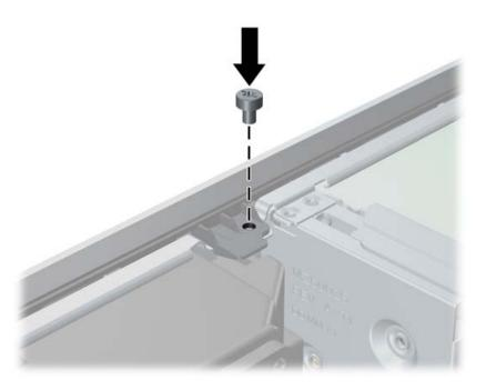
To remove the front bezel security screw, reverse the installation procedures.
