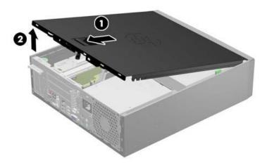
To install the computer cover, reverse the removal procedure.
