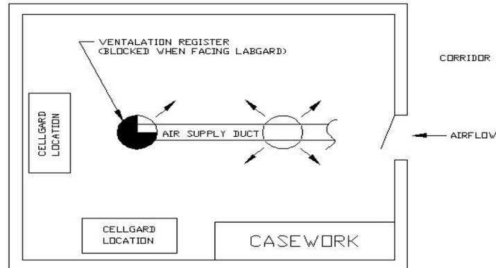
If drafts or other disruptive air currents exceed the inflow velocity of the cabinet through the access opening, the *potential* exists for contaminated air to exit or enter the work zone area of the cabinet. It depends on the severity of the air current. Since this cabinet is mobile, disruptive air currents should be evaluated in each potential cabinet location.
