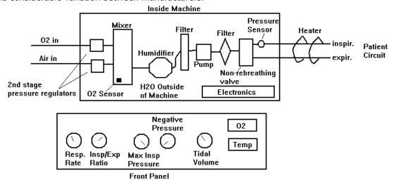
Ventilators are complex devices. In many cases, the only repairs possible in the field are user error, filters and rain out.
