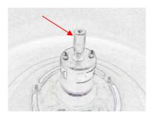
Use the puller supplied with the tool kit to pull off the AutoLock from the motor cone.
