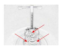
Loosen the center screw completely and remove the AutoLock.
