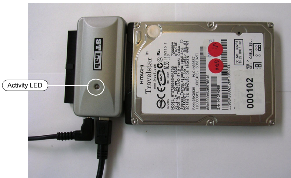
Figure 8-13 PATA Hard Disk Connected to the USB-to-SATA/PATA Adaptor
