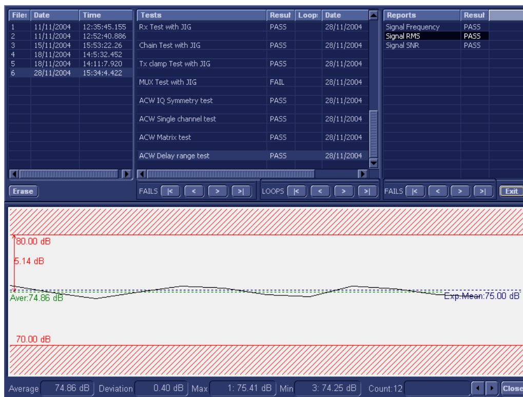
Figure 7-43 View Test Log - ACW Delay Range Test - Signal RMS
