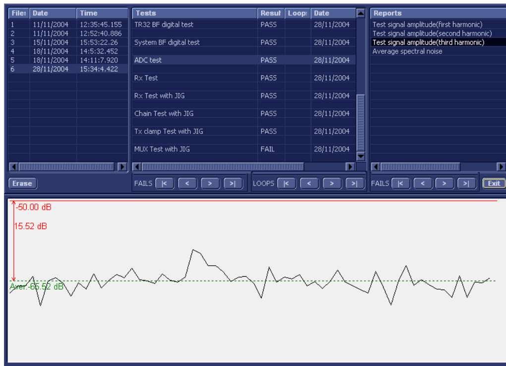
Figure 7-30 View Test Log - Third Harmonic
