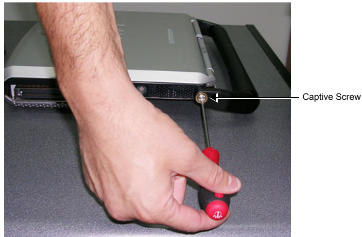
Figure 8-2 Releasing the Bearing Handle Captive Screw
