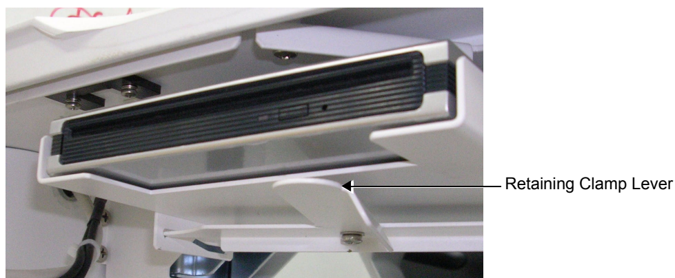
Figure 3-23 Retaining Clamp for DVD-R/RW Drive
