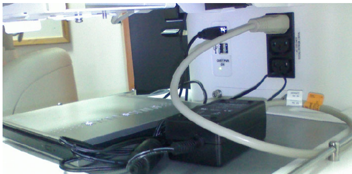
Figure 3-22 Samsung DVD/CD-RW Drive Connected through 5V Power Supply
