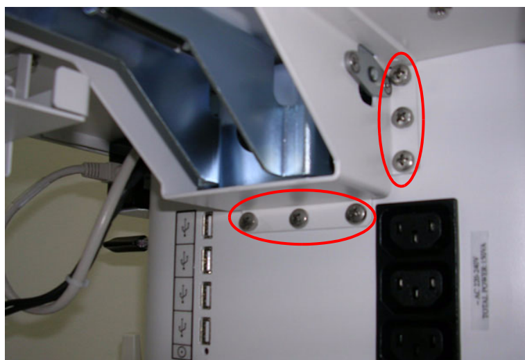
Figure 8-102 Top Shelf - Lower Retaining Screws
