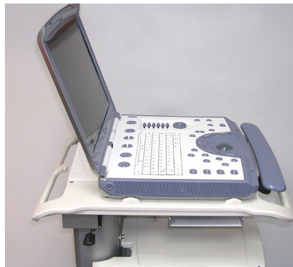
Figure 3-70 Vivid-i™ Scanner Mounted on SafeLock Cart
