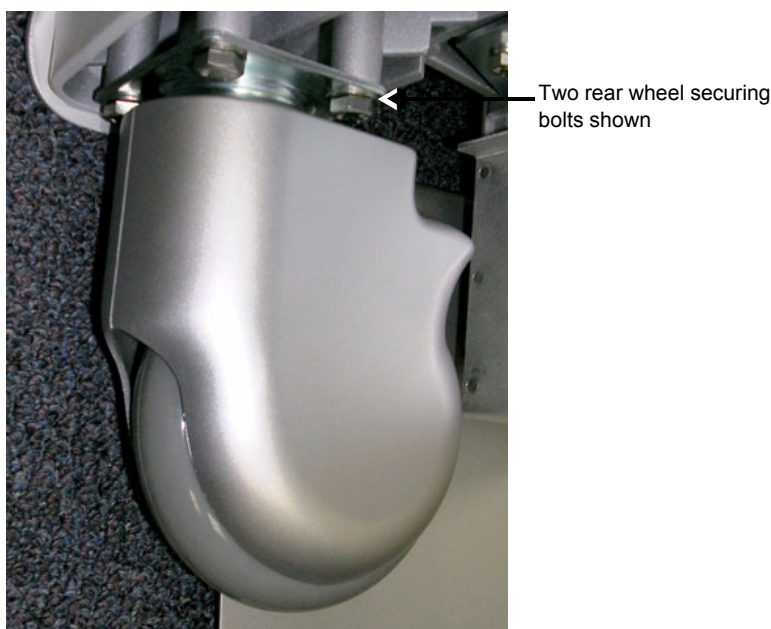
Figure 8-109 Rear Wheel Bolted to SafeLock Cart Chassis
