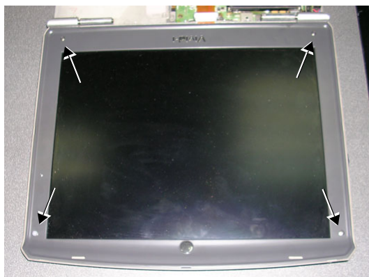
Figure 8-38 Removing the Securing Screws
