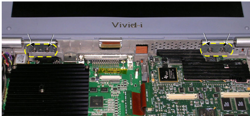
Figure 8-34 LCD Display Hinges Secured to Base Assembly - Location of Screws
