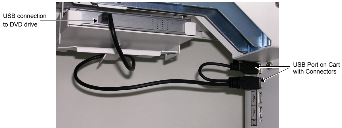
Figure 3-25 USB Cable Plugged Into the DVD/CD Drive and the Cart's USB Connectors
