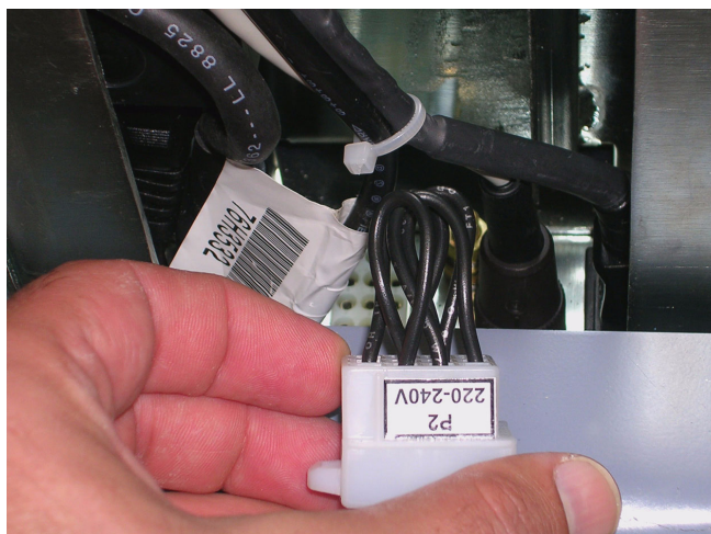
Figure 3-17 SafeLock Cart (Old-type) Voltage Setting
