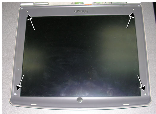
Figure 8-69 Removing the Screws from the LCD Display
