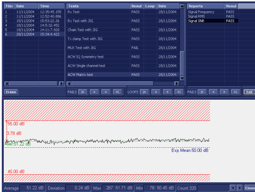
Figure 7-40 View Test Log - ACW Matrix Test - Signal SNR
