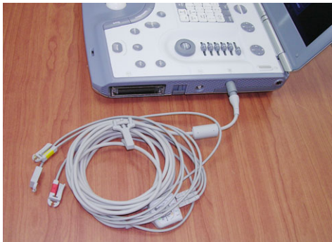
Figure 3-65 ECG Cables Connected to the ECG Connector Port
