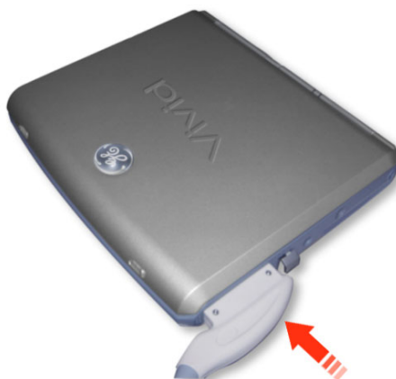
Figure 3-63 Connecting Probe to the Vivid-i™
