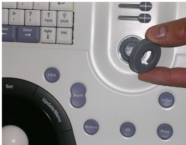
Figure 8-28 ATGC Rotary Knob Replacement
