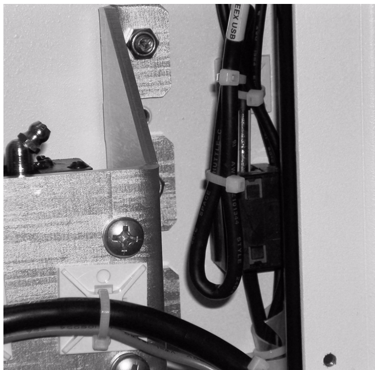
Figure 8-93 USB Power Cable Folded and Fastened with Tie-wraps
