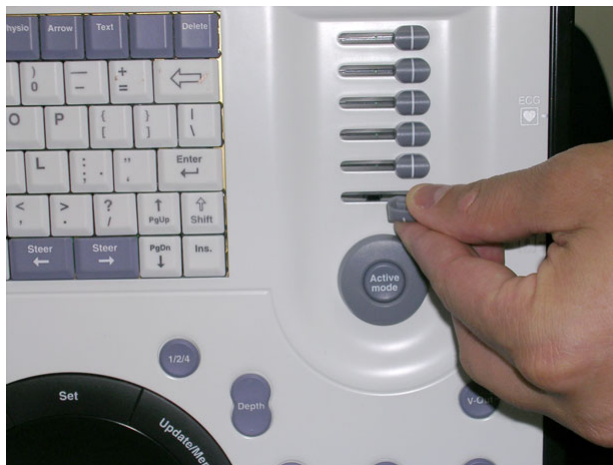
Figure 8-27 ATGC Slider Keycap Replacement
