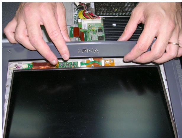
Figure 8-39 Removing the LCD Display Frame
